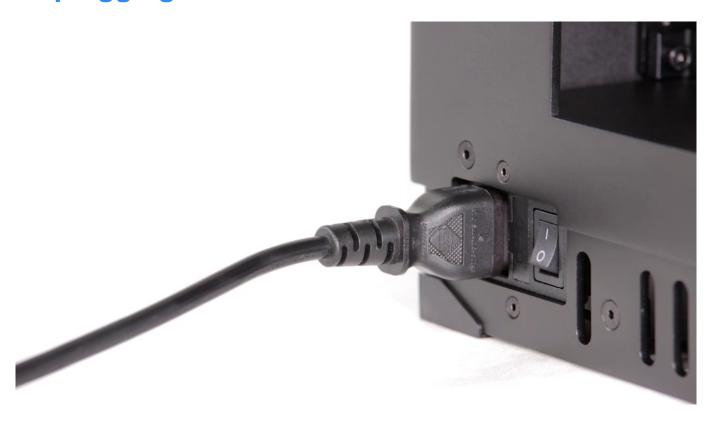
Turn off the printer and unplug the power cable. Wait about 15 minutes and let the machine cool down.
