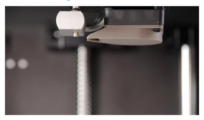
Install the new nozzle in the hotend and screw it in clockwise using the nozzle key (when viewed from below).
