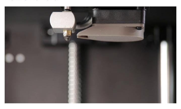
Unscrew the nozzle counterclockwise (when viewed from below). Use the nozzle key from the Starter Kit box. Removing the nozzle should take place while the extruder is still hot. When the nozzle is loose, remove it using pliers.
