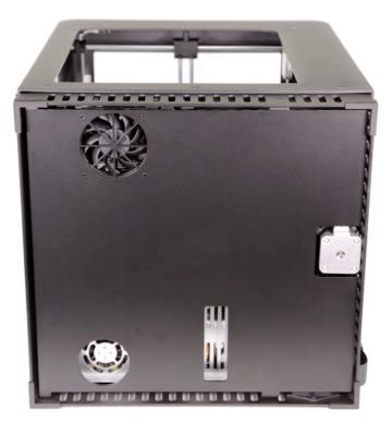
Unscrew the screws that secure the bottom plate on one side of the housing. Use a 2.5mm Allen key.
