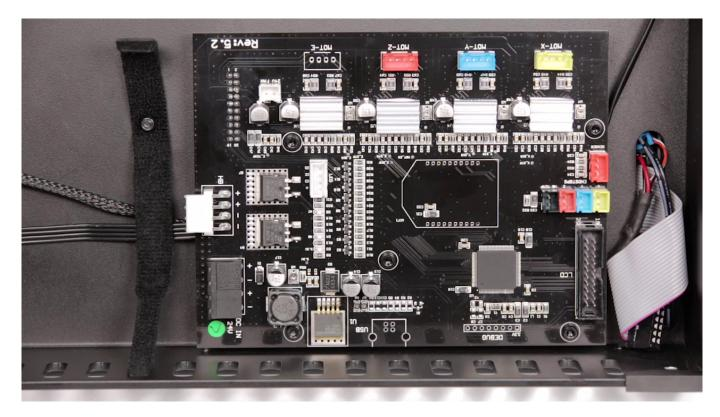
Unscrew the five screws that secure the motherboard using a 2.5mm Allen key and remove the motherboard from the printer.
