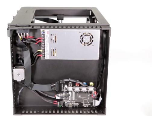
Plug the bottom fan cable into the motherboard and install the bottom plate.
