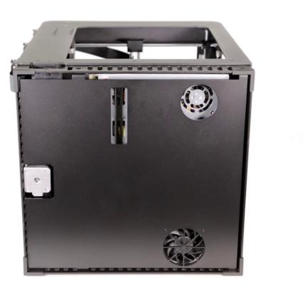
Separate the bottom plate from the printer and unplug the bottom fan cable from the motherboard.
