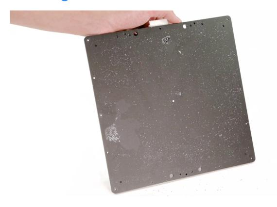
Remove material residues from the heatbed using a piece of cloth or, if it is necessary, use a spatula.
