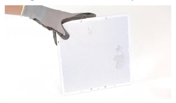
Turn the perforated plate over and clean it from material remains using a spatula.
