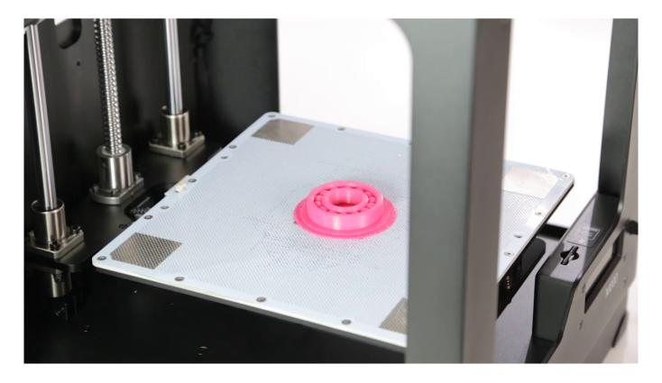
Remove the platform from the printer.
