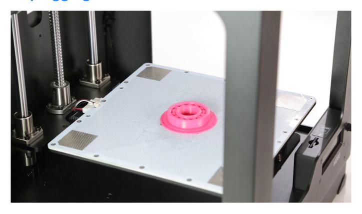
Unplug the heatbed cable from the platform. Both the big and small connectors need to be unplugged.
