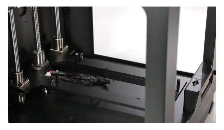
Put the platform back in the printer and plug the heatbed cable in. Both big and small connectors need to be plugged in.
