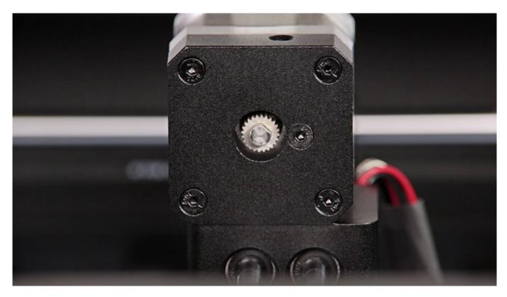
Unscrew the four screws that secure the extruder motor.
