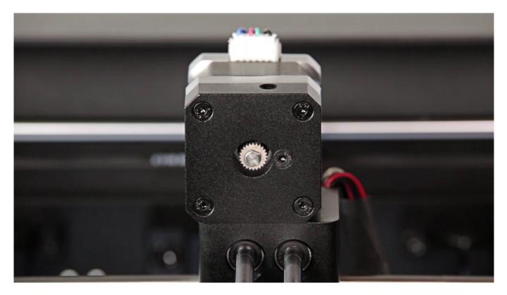
Reattach the extruder aluminum cover to the extruder and secure it with the screws.
