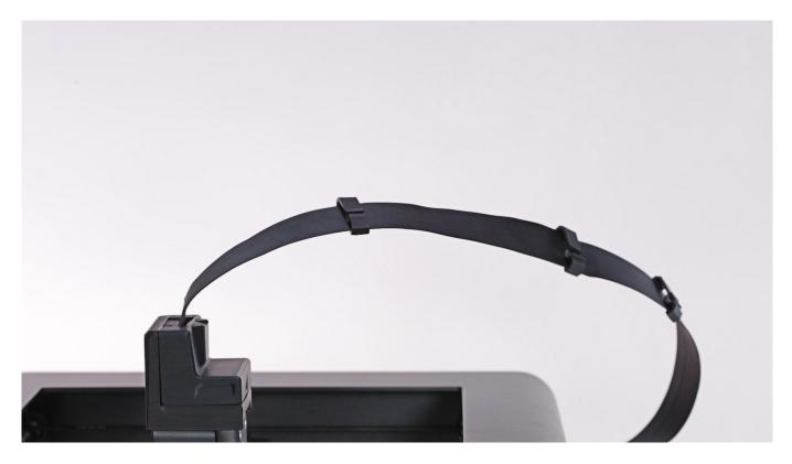
Attach the material guide to the extruder cover. Next, secure the guide to the extruder cable with the material guide clamps.
