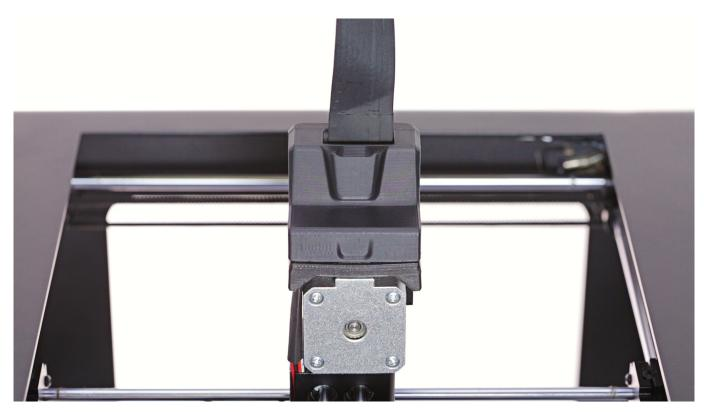
Detach the extruder upper printed cover and unplug the extruder cable.
