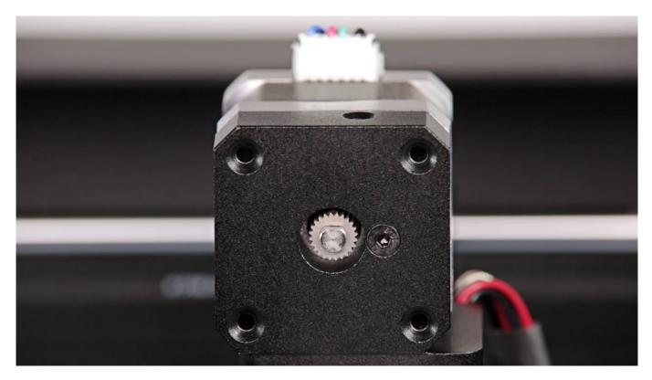
Separate the extruder motor from the extruder block.
