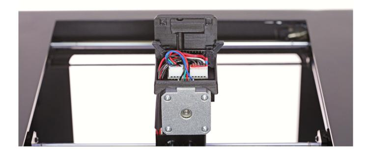
Plug the extruder cable in, and then attach the extruder upper cover to the lower cover.
