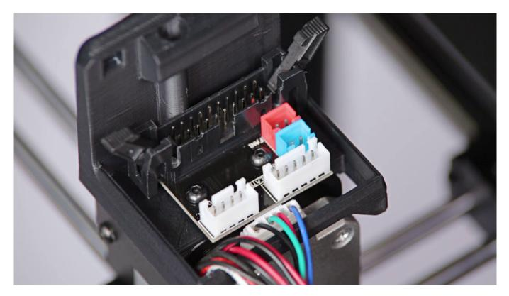
Plug all the cables in. Remember to arrange the cables so that they don't get damaged, e.g. by wrapping against each other.
