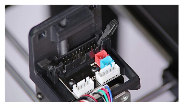
Unscrew the two screws that secure the extruder PCB using a 2mm Allen key. Remove the PCB from the extruder.
