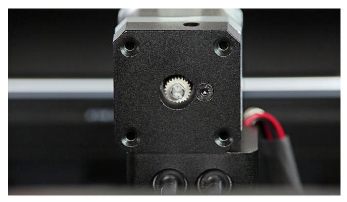
Secure the motor with the screws. Press the motor to the right side so that the bearing rack is as close to the bearing as possible. Tighten the screws crosswise in the following order: 1-4, 2-3.
