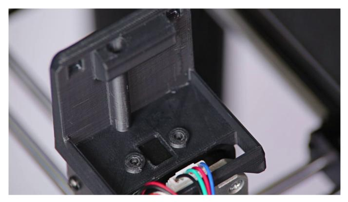
Place the extruder PCB in its place and secure it with the two screws.
