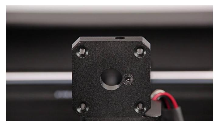
Reattach the extruder motor to the extruder block.
