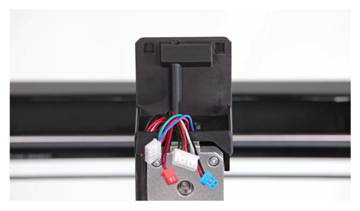
Remove the extruder lower printed cover.
