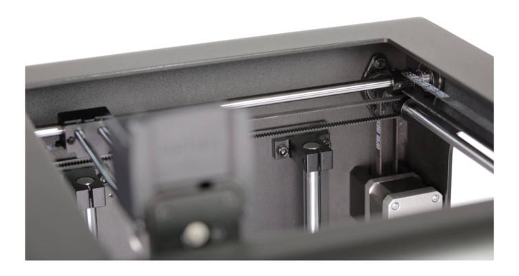
There are 2 drive pulleys on each axis, which are placed next to the long belts (8 drive pulleys altogether). Each pulley has two screws. Tighten each screw on each drive pulley (16 screws altogether).
