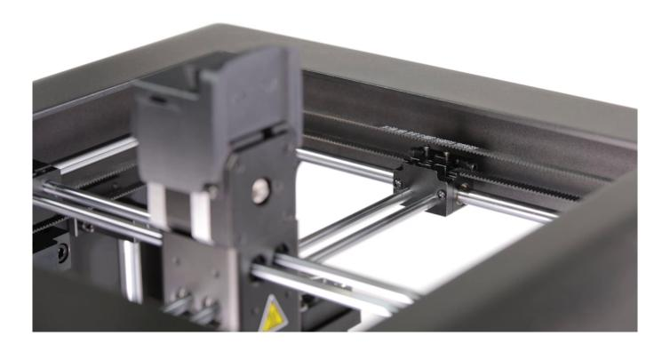
Move the extruder to the center position. Tighten the screws on the axis block using a 1.5mm Allen key.
