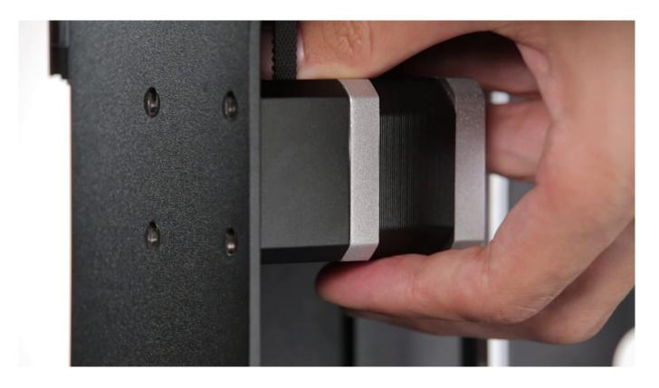
Remove the motor distance piece and remove the motor.
