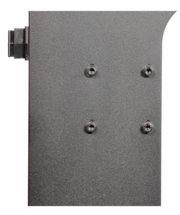
Unscrew the four screws that secure the motor using a 2.5mm Allen key.
