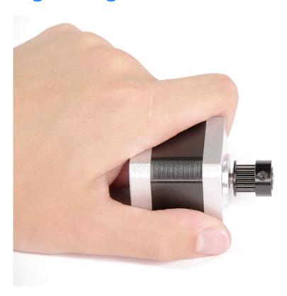
Tighten the screws on the motor pulley using a 2mm Allen key.
