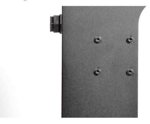
Loosen the four screws that secure the motor using a 2.5mm Allen key.
