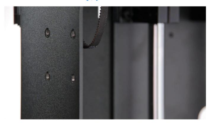
Put the belt on the motor pulley and install it with the distance piece.
