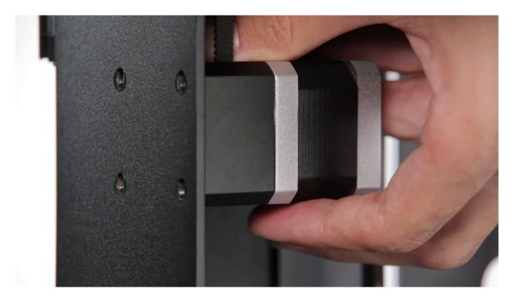
Remove the distance piece and remove the motor.
