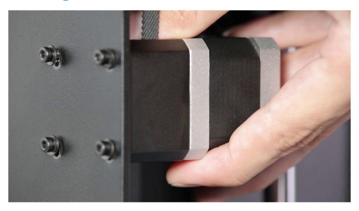
Press down the motor by hand to tense up the belt. Tighten the screws while the motor is still being pressed down.
