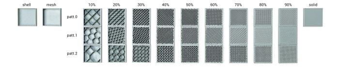
The infill option determines the amount of material that will be printed within the walls of the model. This option influences the model's durability and weight, both of which can be increased by setting a higher level of infill. However, the higher infill, the more time and material will be needed for such a print.
