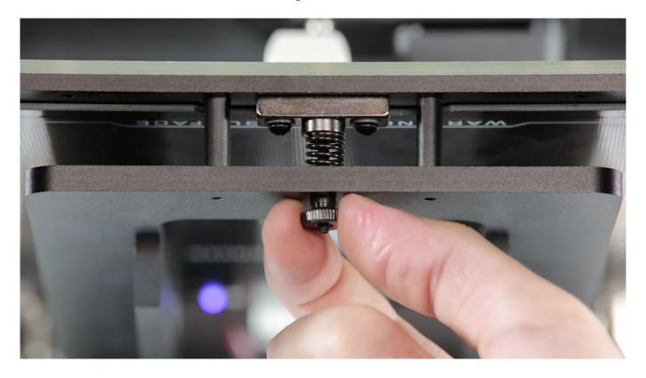
Platform calibration involves a procedure of checking the distance between the nozzle and five calibration points on the platform, and tightening/loosening the calibration screws.
