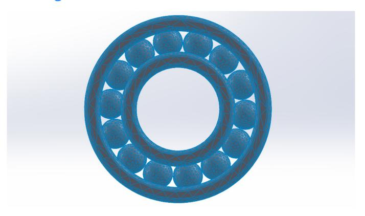
While printing movable parts, it is importrant to keep proper spaces between particular parts. These spaces are responsible for the flexibility of your model. The minimum space requirement is 0.4mm for these kinds of prints.
