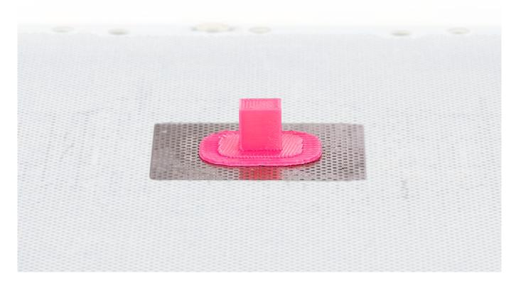
Very small objects require some additional options such as the appropriate FAN SPEED and LAYER THICKNESS settings.
