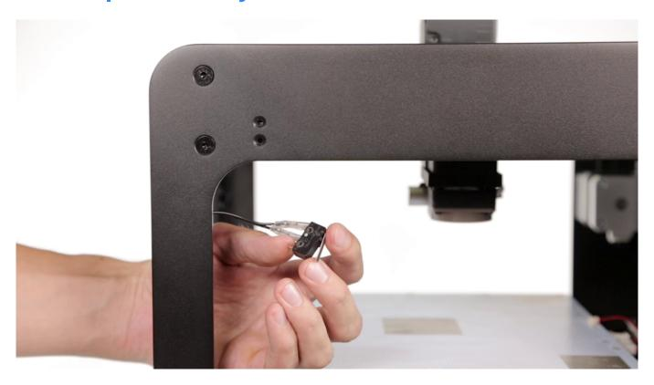
Install the new endstop in its place and secure it with the screws.
