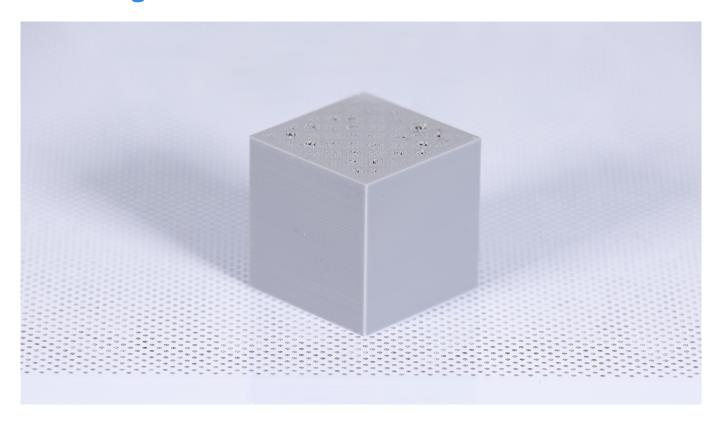
Pillowing is another problem mainly caused by improper settings in Z-SUITE. This effect is always visible on 3D models with flat surfaces and low infill. The top surface can be uneven, and have bumps or sometimes holes in it. You can experience this effect on your models after setting too few top and bottom layers in Z-SUITE.
