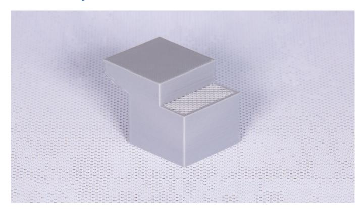
If layers on your model become shifted during the printing process, you need to carry out some maintenance work connected with the axes. This printing issue is caused by loose pulleys on the X or Y axis motor.
