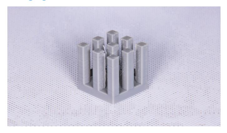
Another undesired effect of overheating is called stringing or, in other words, "hairy prints." Stringing is especially visible on models with thin parts that are arranged at a certain distance from one another. This effect occurs when the material becomes too liquid due to overheating, and it leaks through the nozzle when the extruder is making a non-print movement.
