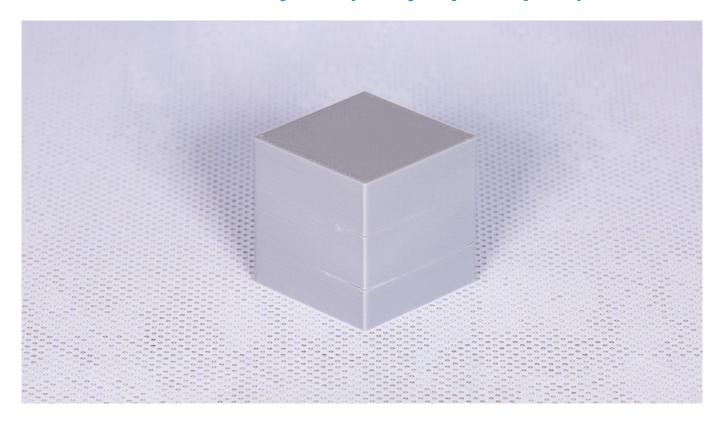
Good printing conditions are very important for a model's good quality. Always print in a room with little air flow, at a stable room temperature. Layers of material need proper temperature to stick to one another.
