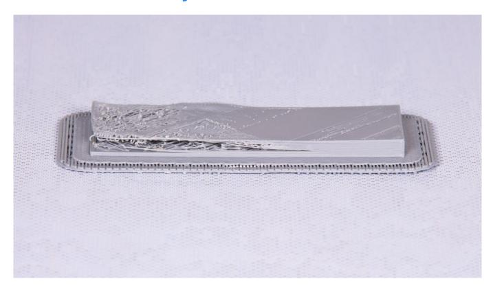
Technical problems are common causes of serious printing issues. Worn or damaged replacement parts can have a negative influence on the final look of a model. For example, a damaged extruder cable will cause extrusion problems.
