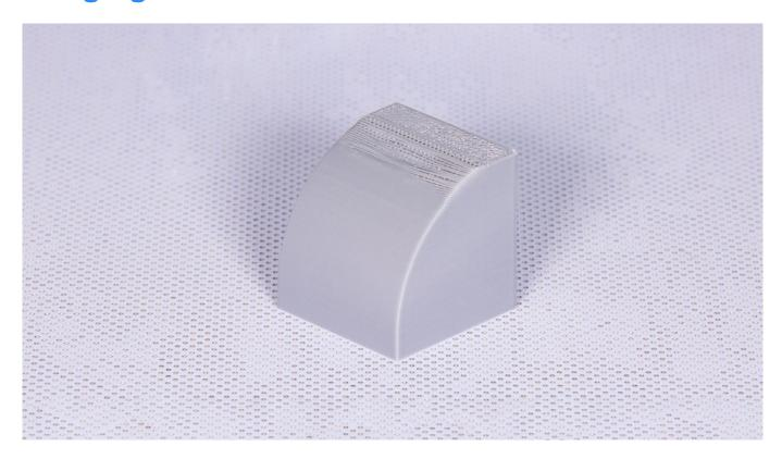
Inadequate settings can cause another issue with 3D printed models. There are a few settings in Z-SUITE that you need to adjust to avoid the problem of hanging strands on a model: *Support*, *Layer thickness* and *Fan speed*.
