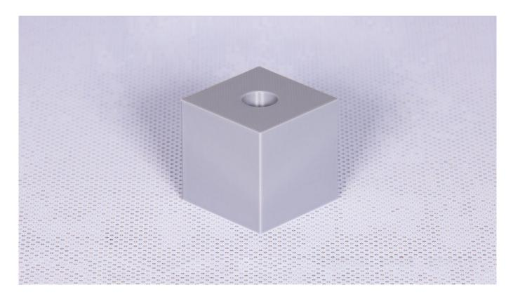
While designing holes in your model, you have to keep in mind that the designed hole should be bigger than the one which will be printed. The hole should be  $\sim$ 0,3mm bigger than the one you want obtain.
