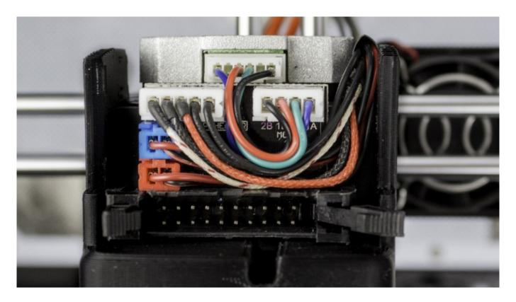
If you can hear a clicking sound coming from the extruder motor during the material loading or printing, at first check if all cables are properly connected to the extruder PCB. See the picture.
