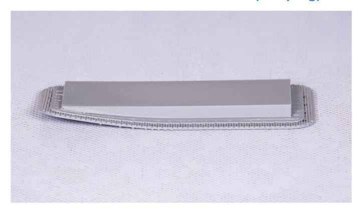
The first few layers of material, which begin the whole printing process are called RAFT. These layers are always printed before the main object and have a larger area than that object. Once the printing is done, the RAFT needs to be removed from the platform together with the rest of the model. The raft enhances the adhesion of the whole print to the platform and reduces the risk of warping.
