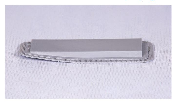
The first few layers of material, which begin the whole printing process are called RAFT. These layers are always printed before the main object and have a larger area than that object. Once the printing is done, the RAFT needs to be removed from the platform together with the rest of the model. The raft enhances the adhesion of the whole print to the platform and reduces the risk of warping.
