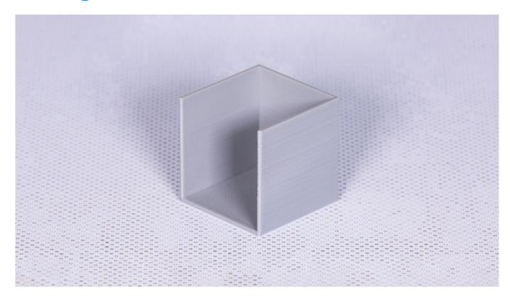
If there are missing walls in the structure of your model, it means that the model has been poorly designed – the walls in the X and Y axes should not be less than 0.4mm.
