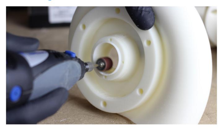
If the residues are difficult to remove, use a grinder to smooth down the surface of the model.
