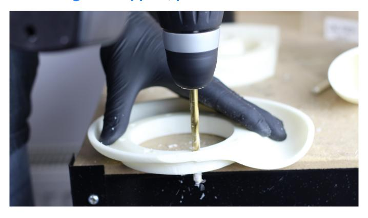
If there are any holes in your print, remove the support from them using a drill or a drill-driver.
