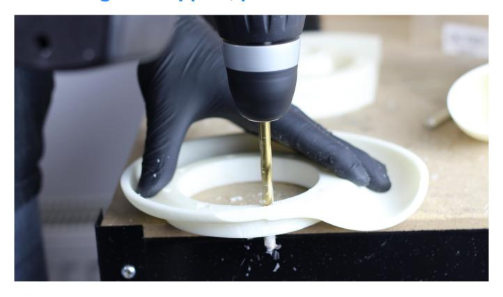
If there are any holes in your print, remove the support from them using a drill or a drill-driver.
