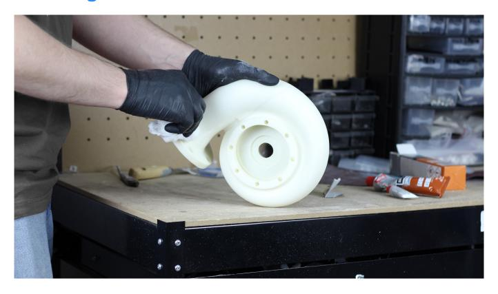
Clean the surface of the print with petroleum ether to prepare it for spackling. Make sure that the surface is free from oil and dust. It is an important step because the residues of dust, oil and other dirt may damage the final effect. Petroleum ether dissolves the residues without damaging the material that the print is made of.
