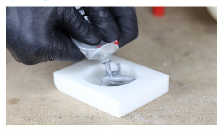
Use spackling paste for plastics to fill the gaps in your print. Mix the paste in a container until you get a smooth and lump-free texture.
