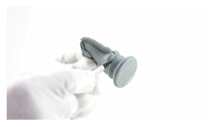
Use the scalpel from the Starter Kit box to remove the remaining support.
