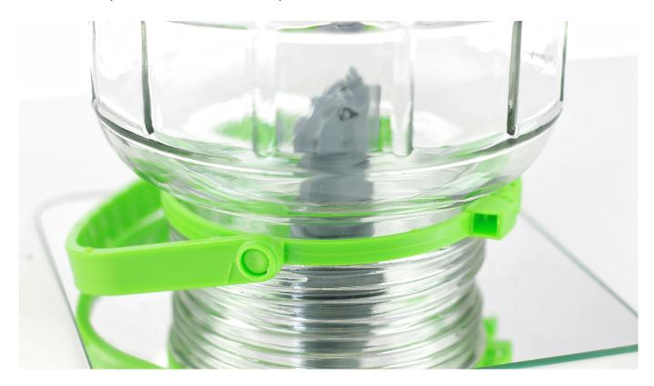
Cover the model with the jar and leave for about an hour. The model shouldn't be kept under the jar for more than an hour as the acetone vapor may melt the details or damage your print.
