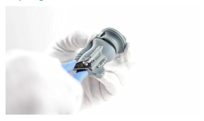
Remove the raft and support using pliers.
