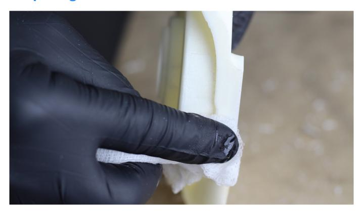
At first you have to prepare the surface of your print for gluing. It has to be rough so as to increase the adhesion of the glue. Use 150 grit sandpaper. Next, clean the surface with a piece of cloth damped with petroleum ether from dust and oil.
