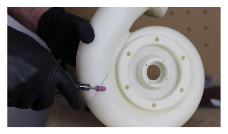
If it is possible, remove dried glue residues with a grinder or a scalpel.
