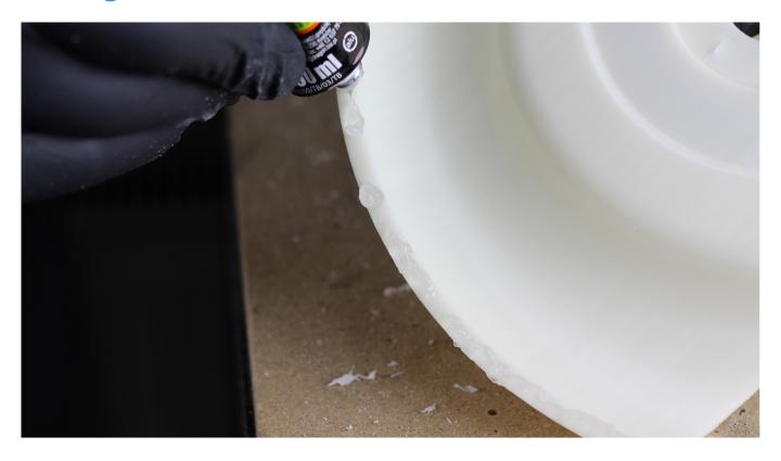
Cover the surface with glue. We recommend using cyanoacrylate glue for plastics.
