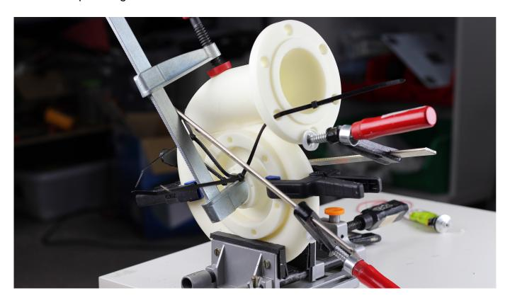
Leave the print for the time required by the producer of the glue. To ensure proper bonding, use clamps which will keep the two parts as close to each other as possible.
