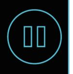
You can pause a print manually at any point of the printing process. Press the knob for **10 seconds** to pause the print. Once you pause the print, additional options will appear on the display:
