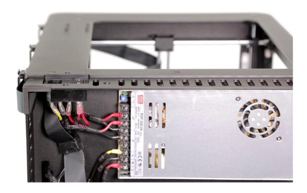
Secure the power switch with the two screws using a 2mm Allen key.
