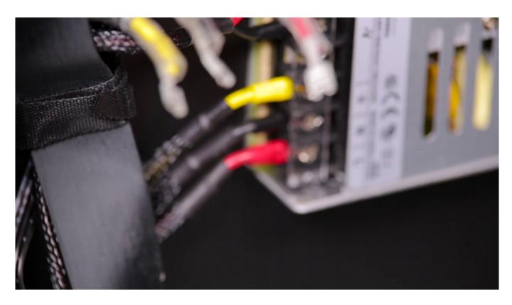
Install the new power switch in the housing, plug all the cables in and put the insulation back on the cables.
