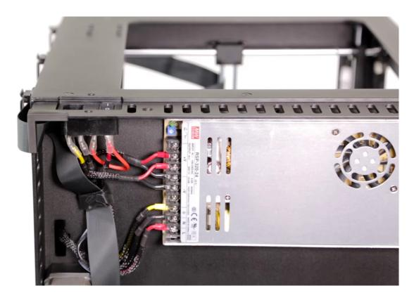
Separate the power switch from the housing, remove the insulation from the cables and unplug all the cables.
