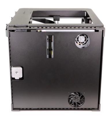
Separate the bottom plate from the printer and unplug the bottom fan cable from the motherboard.
