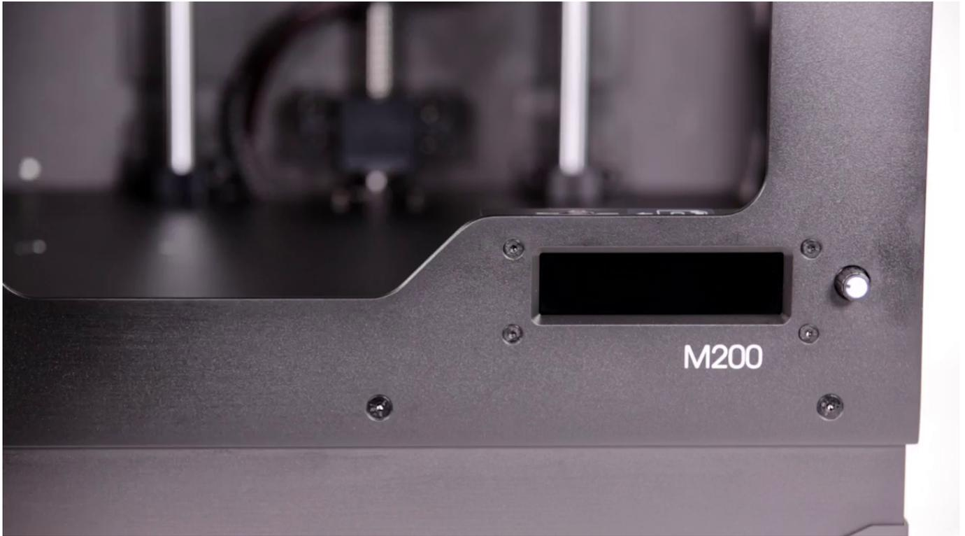
Unscrew the four screws that secure the panel to the front frame of the printer
