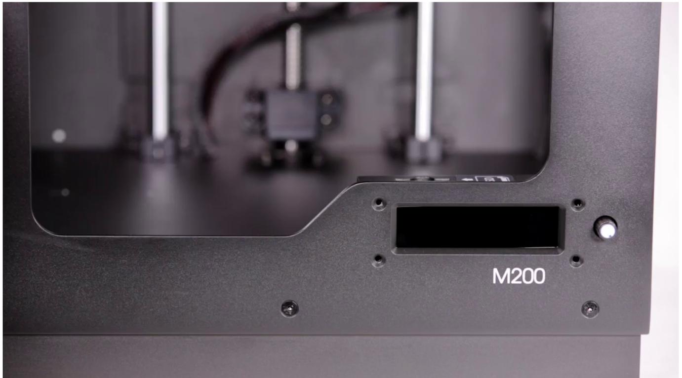
Secure the panel with the four screws.
