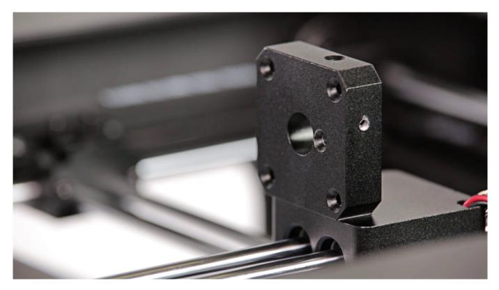
Insert the new bearing into the extruder block and secure it with the screw.
