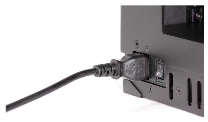
Turn off the printer and unplug the power cable and wait a few minutes for all the capacitors to discharge.
