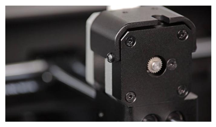
Unscrew the screws that secure the extruder aluminum cover on both sides of the extruder. Separate the cover from the extruder motor.
