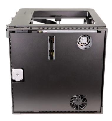
Secure the bottom plate with the screws on one side of the housing. Use a 2.5mm Allen key.
