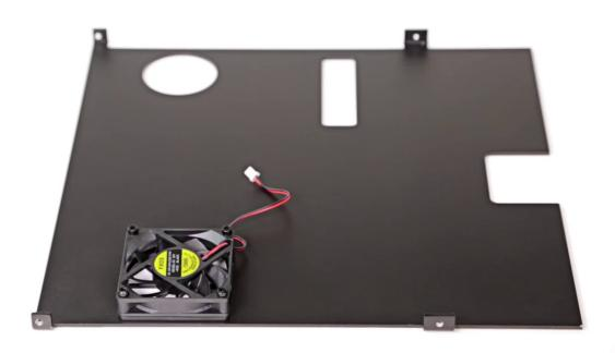
Unscrew the bottom fan from the plate using a 2.5 mm Allen key. Remove the bottom fan cable from the clamp and separate the fan from the bottom plate.
