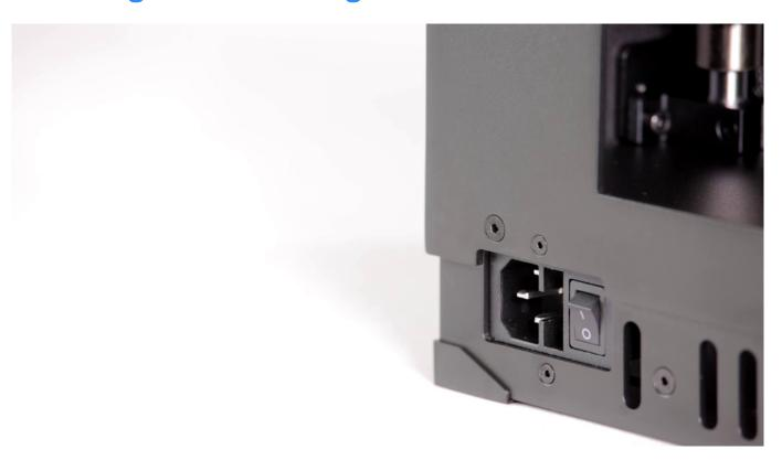
Insert the plug with the new fuse into the slot next to the power switch.
