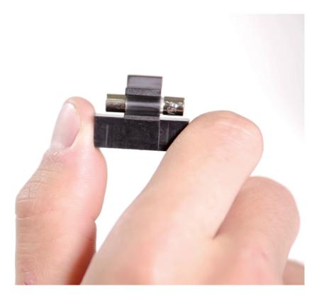
Remove the old fuse and insert a new one: 250V F5AL 5 Amp.
