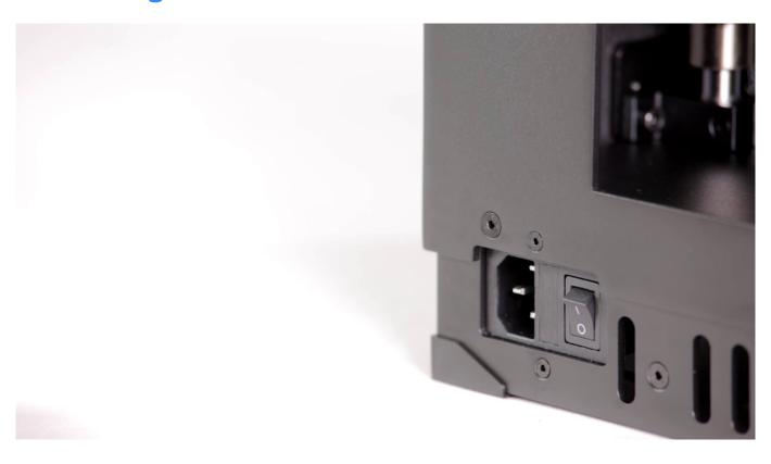
Remove the fuse plug using a flathead screwdriver. The plug is placed next to the power switch.
