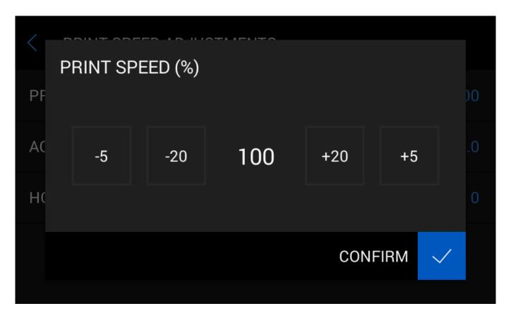
*Print speed* – this is the speed of the extruder head moving in XY axes while printing. The default value is 100%. You can go up to 300%. Remember that the printing speed of raft, infill, supports, contours is not identical, so when you change the print speed to 300%, it means that each of them will be printed 3 x faster than their default values
