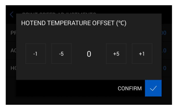
Hotend Temperature Offset – printing in a high speed mode might require increasing the hotend temperature. Faster movements in the XY directions, and having the default hotend temperature, might result in material deficiency on the print. In order to "keep up" with extruding while printing with very high speed, you can increase the extrusion temp. (5 degrees Celsius - more is not recommended)).
