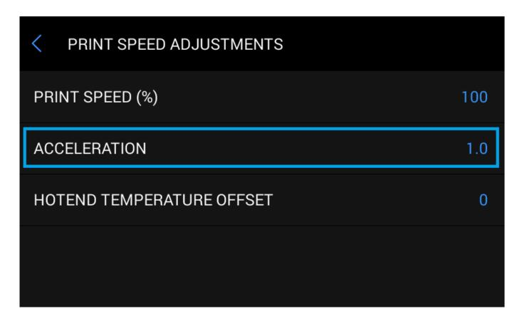
Acceleration – this option determines how fast the extruder accelerates after changing direction of printing. It can gain the speed slowly or more rapidly. The values are: x0.75, x1.0, x1.5, x2.0. The default one is x1.0. We recommend using x1.5.
