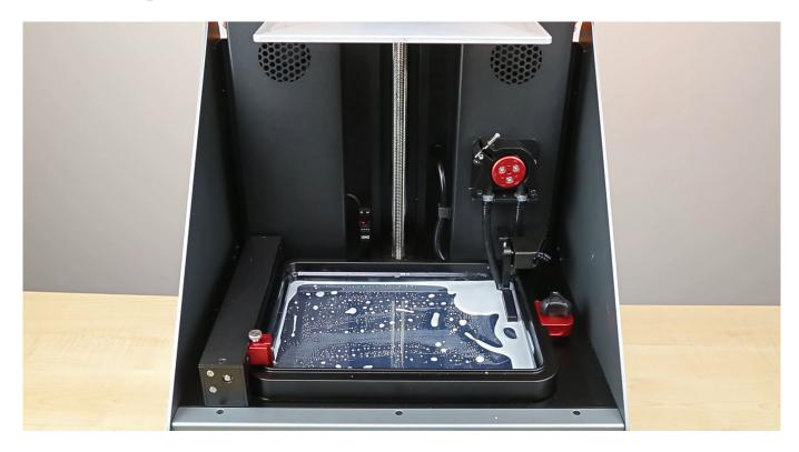
The printer will now start pumping the IPA solvent into the resin vat.
