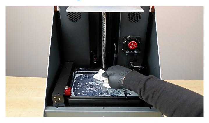
Clean the resin vat from remaining resin using paper towels. Make sure not to damage the FEP film. Once you cleaned the vat, click *Continue*.
