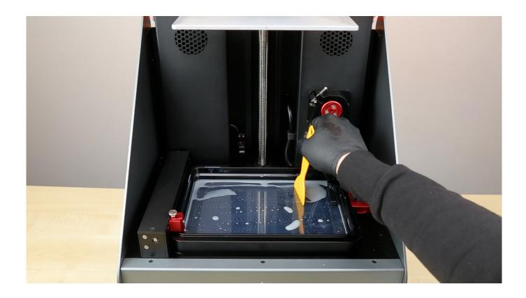
At the stage 5 of *Pumping Out*, you can use the plastic spatula included in the Starter Kit in order to help remove the remaining solvent. Make sure not to damage the FEP film.
