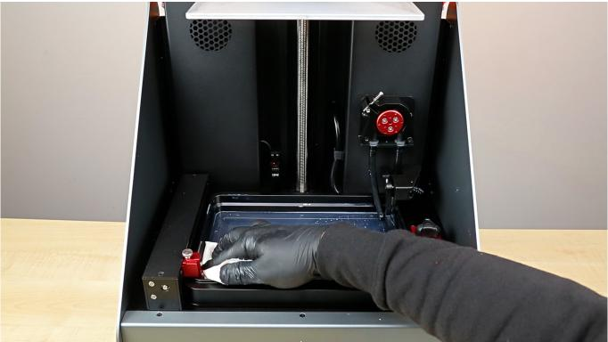
Use a paper towel to gently clean the resin vat from remaining solvent. Make sure not to damage the FEP film. When done, click *Continue* on the screen.
