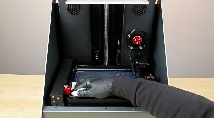
Use a paper towel to gently clean the resin vat from remaining solvent. Make sure not to damage the FEP film. When done, click *Continue* on the screen.
