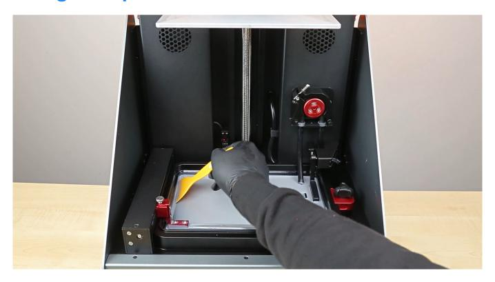
Use the plastic spatula included in the Starter Kit to help remove the remaining resin. Direct the resin towards the tube. Make sure not to damage the FEP film.
