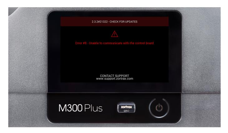
The picture shows a firmware message that indicates an Android PCB-motherboard communication problem. Once you receive this notification, follow the steps from this manual.
