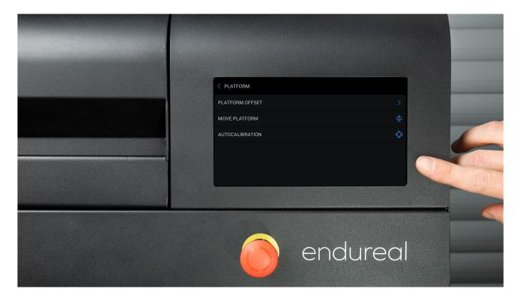
Calibrate the platform. Open the *Tools* menu and select *Platform*, and *Autocalibration*. Follow the instructions displayed on the screen.
