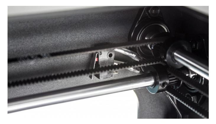
Check if the endstop cables are properly plugged into each endstop.
