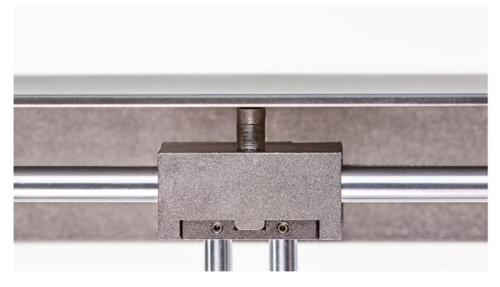
First, check if the endstop sleeves are installed on each axis block. Make sure the sleeves are not worn out. More details are available in the <u>Endstop sleeve installation</u> manual.
