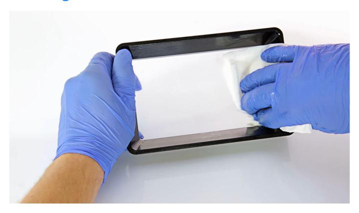
Thoroughly clean the resin tank and FEP film using a paper towel soaked in isopropyl alcohol. If there is cured resin on the film, remove it with a plastic spatula. More details are available at: resin tank cleaning.
