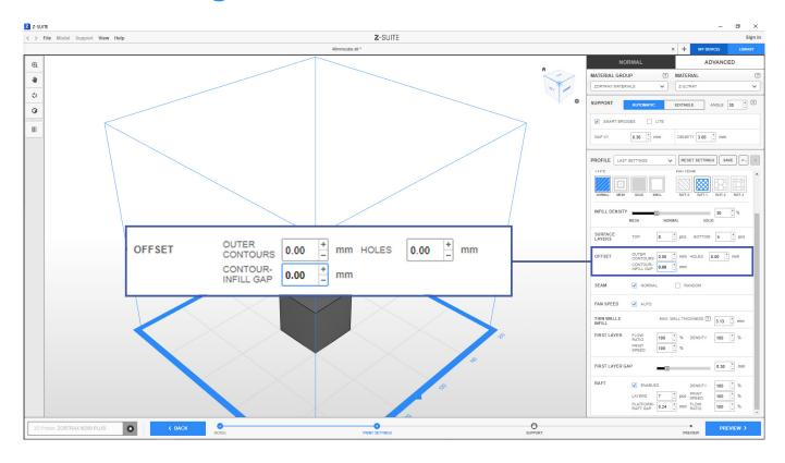
You can counteract the problem with contours at the stage of preparing your model for 3D printing. In the *Print settings* step, open the *Advanced* menu and go to the *Offset* section. Next, decrease the *Contour-infill gap* value. The default contour-infill gap value is 0.4 mm.
