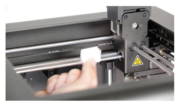
If after the start-up there are problems with axes movement in your printer, apply a thin layer of silicone oil delivered in the Starter Kit onto the axes and carry out the following maintenance procedure: <u>Troubleshooting: Layer shifting</u>.
