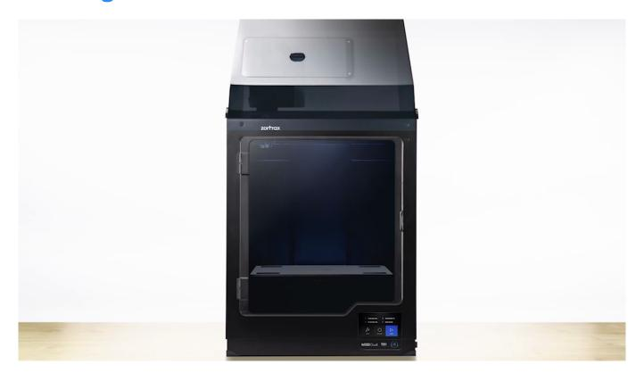
First of all, printing with Z-PETG and Z-GLASS requires providing proper conditions in the print room. The temperature should not exceed 28° C [82° F]. When preparing a file for 3D printing in Z-SUITE, make sure to always check the *Auto* box in the *Fan speed* section. It is not advisable to adjust the Fan speed manually.
