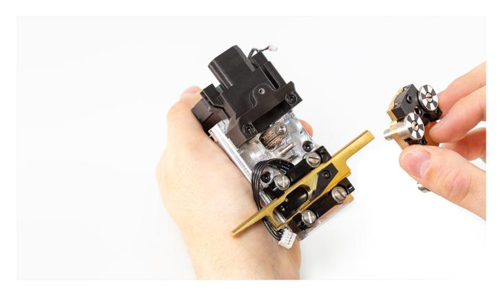
Once you notice that extrusion in your printer is not as effective as it should be, make sure that the model material nozzle and hotend are not clogged, and if it is necessary, clean both components.
