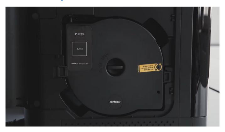
To prevent further printing problems, unload Z-PETG or Z-GLASS immediately after the printing process. The materials should not be left loaded in the hotend as they become more difficult to extrude after some time. Additionally, once you finish printing, print a small-sized object using Z-ULTRAT (or ABS) to remove residues from the nozzle and hotend that can accumulate during when printing with Z-PETG or Z-GLASS.
