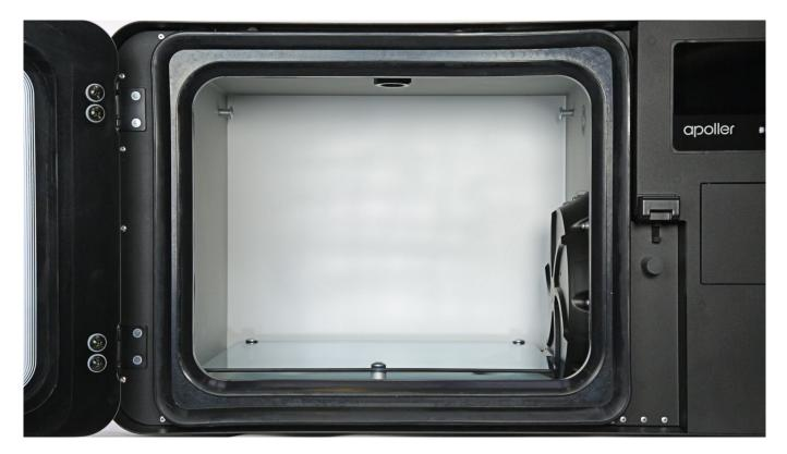
Soak a piece of cloth in acetone or butanone (MEK) and thoroughly clean the chamber door gasket, directing the cloth along the gasket's profile. Remember that the gasket cannot be cleaned with the use of sharp tools.
