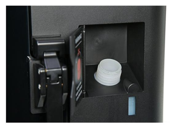
First, remember to properly tighten the filler cap every time you unscrew it to refill or empty the solvent tank. Make sure the cap is properly attached and then tightened with the special key.
