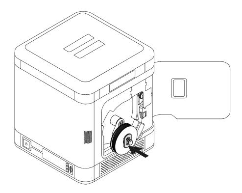
Insert the stopper onto the holder.
