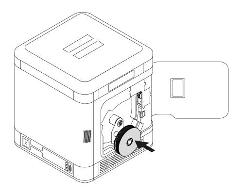
Place the spool on the holder. The spool should rotate anti-clockwise.
