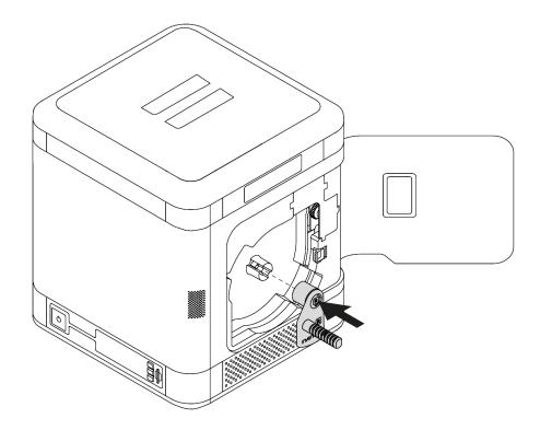
Open the right door by pressing the release buttons. Insert the holder into the slot.
