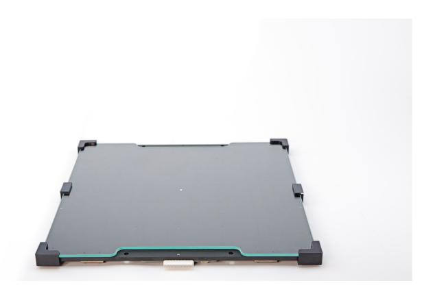
When using a spray adhesive, at first unplug the heatbed cable and remove the platform from the printer. Remember that the spray has to be applied while the platform is cool. Spray the plate from a distance of 15-30 cm [5.9-11.8 in]. Next, wait until the solvent evaporates before installing the platform back in the printer.
