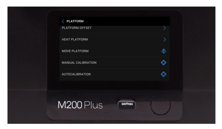
Before you start to print without the raft, you have to properly calibrate the platform in your printer. This procedure makes it less possible for prints to deform during the printing process. When using the glass plate, you have to carry out the manual calibration. It involves adjustments of the platform's position in relation to the nozzle by tightening or loosening the platform screws.
