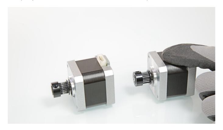
Disassemble the other axis motor (which is probably functional) and check its pulley. Turn pulleys in both motors and compare the way they turn.
