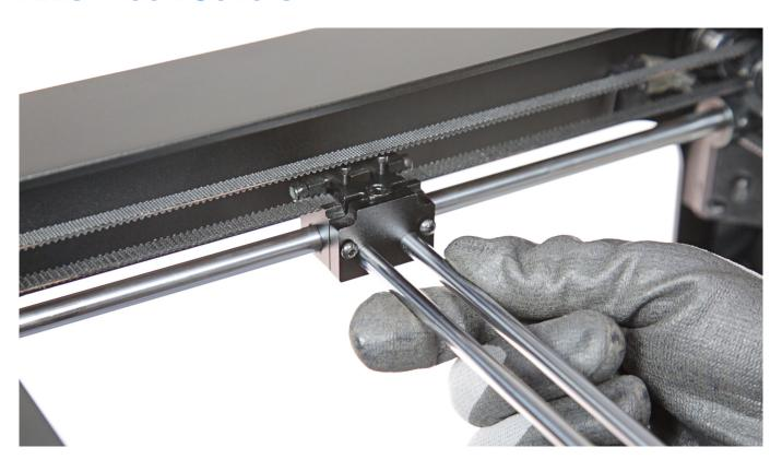
Next, grab the extruder guide rails and slightly move the axis block on the axis in which layers in the print have shifted. In this way, you can check if the block cover is properly secured.
