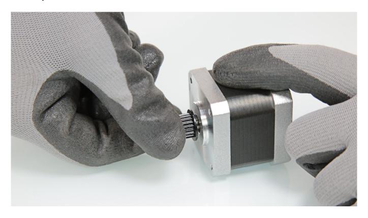
If the pulley rotates with resistance, move on to the next step.
