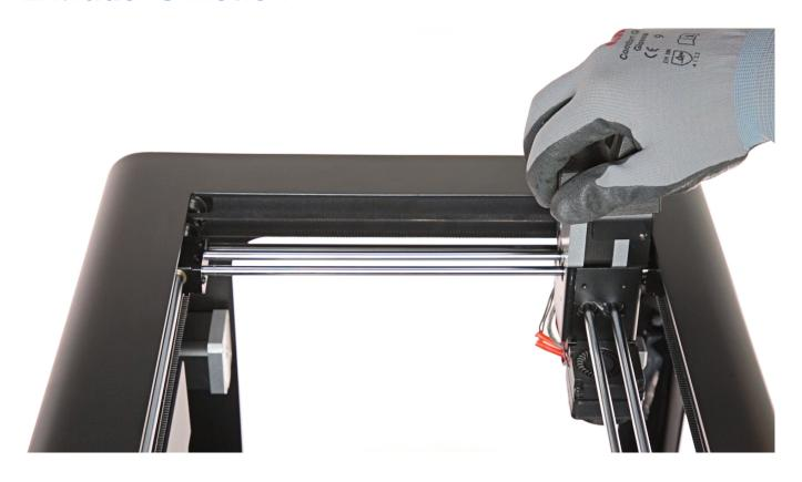
At this point, you have to check if there is resistance when moving the extruder. Turn the printer off and move the extruder manually towards each corner of the housing.
