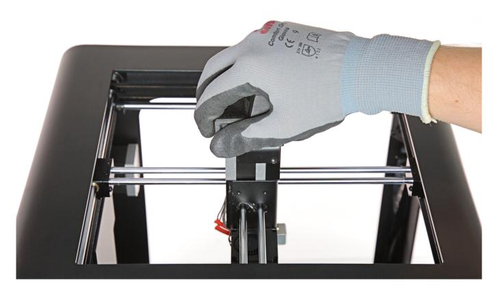
You also have to check the overall state of the belts on the axis that may be causing layer shifting.
