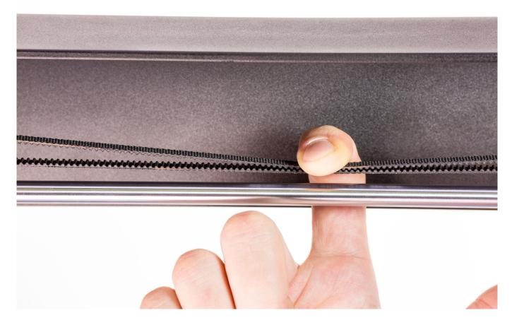
Once you determine the direction of layer shifting – X or Y axis, check if the belts along that axis are properly set on the pulleys.
