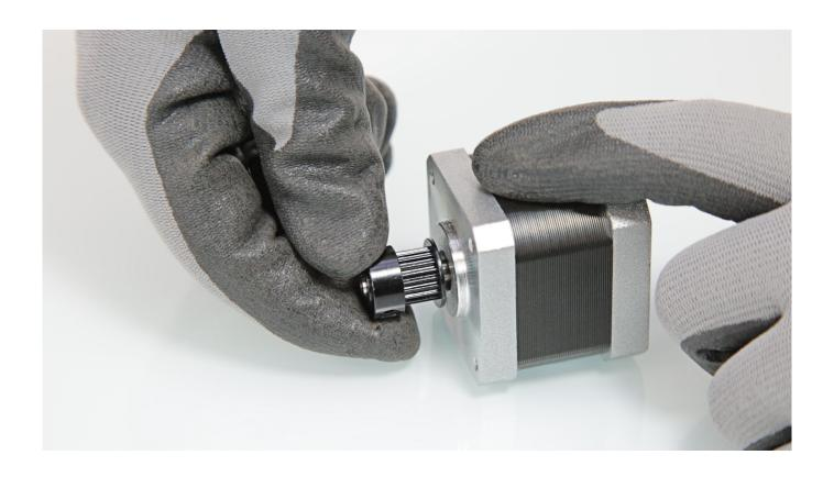
Turn the motor pulley manually to check if there is resistance. The pulley should rotate smoothly.
