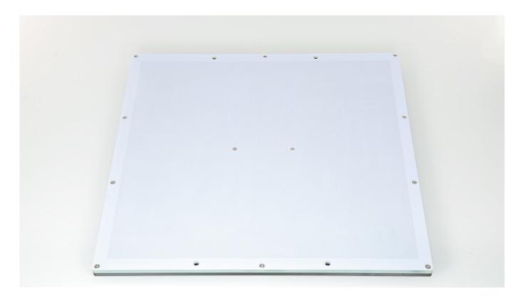
Unscrew the twelve screws that secure the perforated plate to the heatbed. Next, separate the plate from the heatbed.
