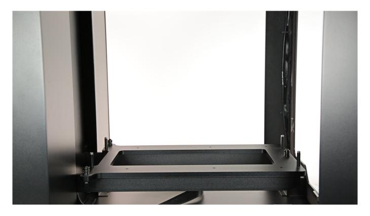
Place the platform in the printer and plug the heatbed cable in. Next, start the platform calibration procedure using the options from the menu\*.
