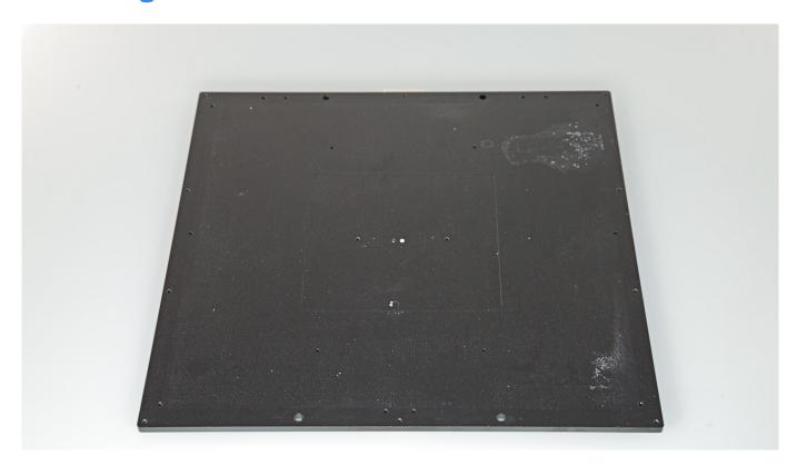
Clean the heatbed from material residues using a piece of cloth.
