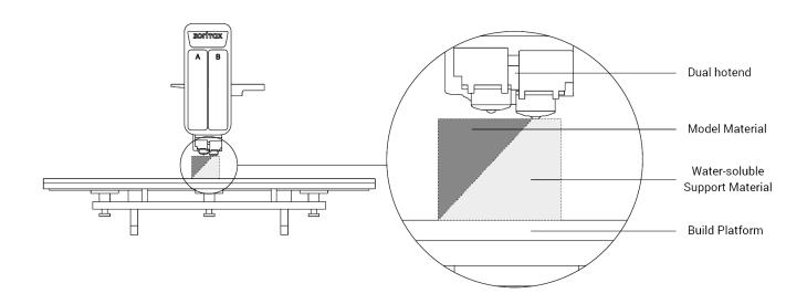
The M300 Dual works in the LPD Plus technology which uses standard thermoplastics and a soluble support material to build 3D parts. This technology involves depositing layers of the two filaments to form a predesigned shape – an accurate representation of a digital model.
