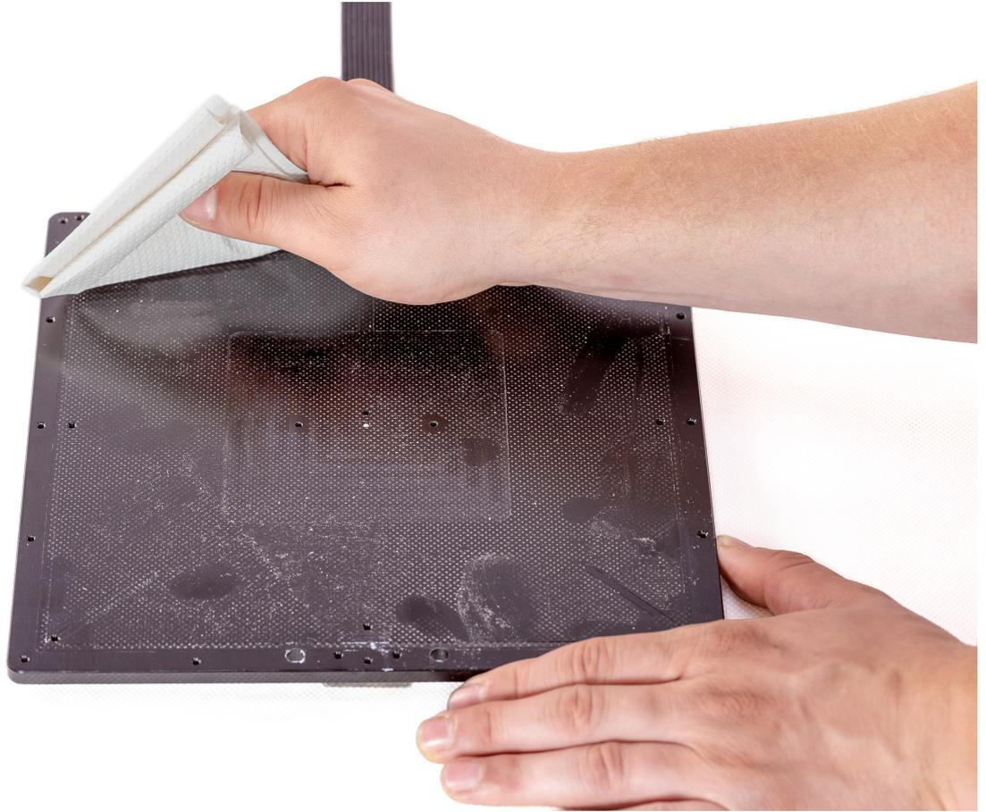
Platform maintenance is another procedure which improves adhesion in your printer. The instructions from the [maintenance manuals](#) will help you while dealing with adhesion problems and other printing issues.
