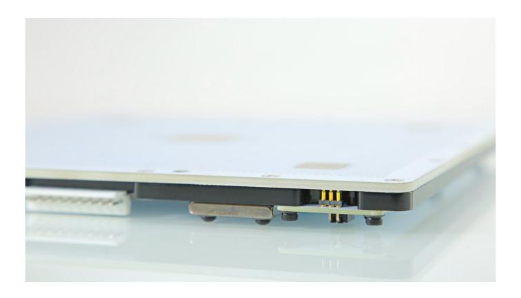
For the M200 Plus, measure the electric circuit continuity between the left pin on the plate's small connector and five calibration squares.
