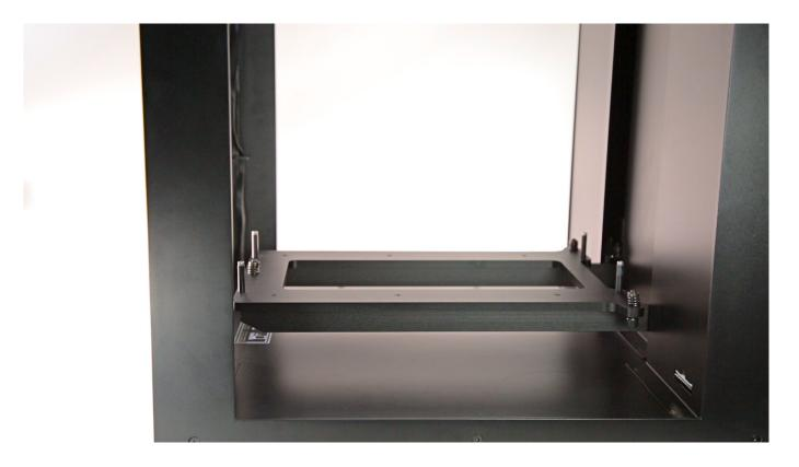
Pass the heatbed cable behind the heatbed mount and install the platform back in the printer.
