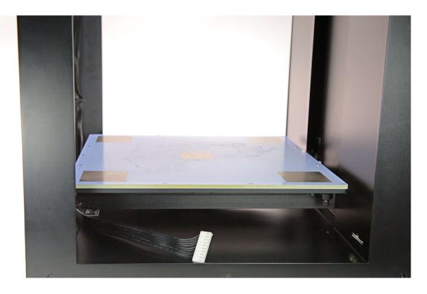
Remove the platform with the heatbed cable from the printer.
