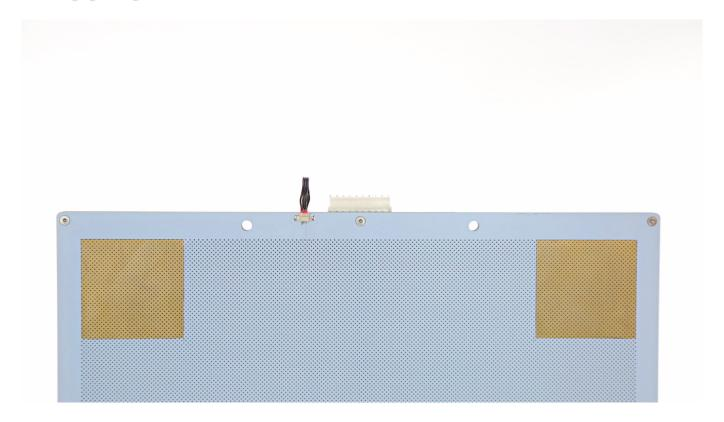
Plug the new heatbed cable into the platform.
