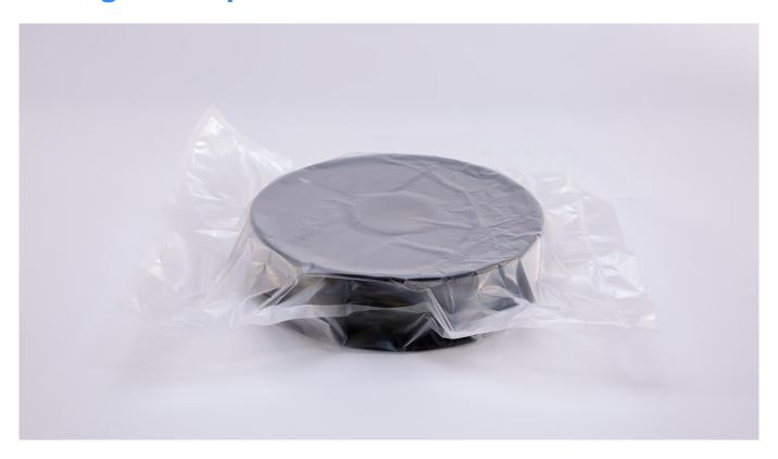
Z-NYLON is highly hydroscopic and shouldn't be stored without protection in humid environments for a long time. Unused spools have to be stored in an airtight container with a moisture absorber. Otherwise, the filament will absorb moisture from air which can cause problems such as stringing or low surface quality of printed parts. Also, the color of the filament can fade or become dull.
