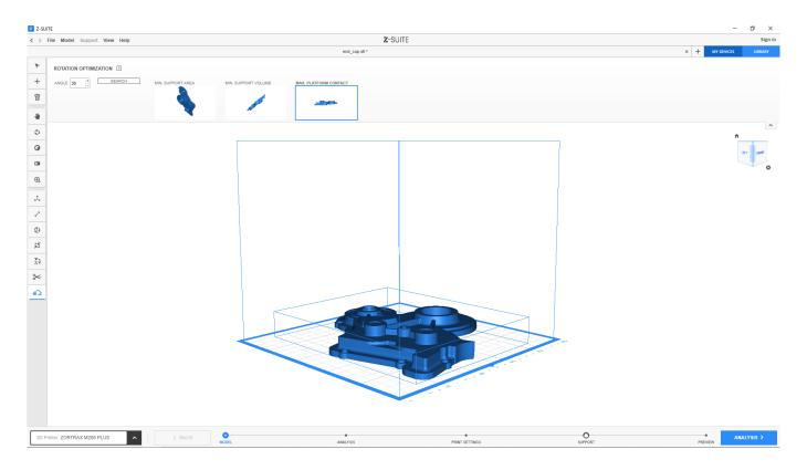
**MAX. PLATFORM CONTACT** – this position places the biggest flat surface of a model directly on the platform. This way big areas which would require a lot of support are eliminated.
