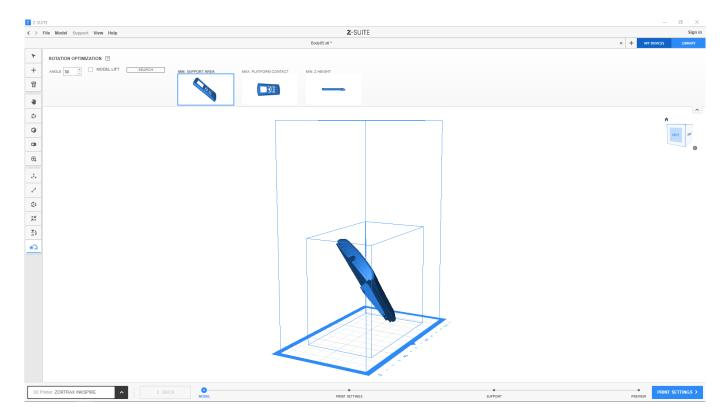
**MIN. SUPPORT AREA** – this position reduces the number of required support structures (pillars). It means that the need of further mechanical treatment is minimized and there are fewer marks on the model's surface after removing the support.
