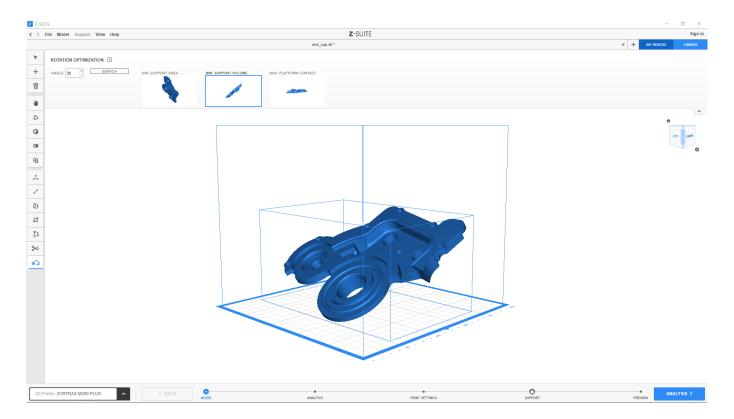
**MIN. SUPPORT VOLUME** – this position allows setting a minimum number of support structures. As a result, the amount of material needed to print a model is significantly reduced.
