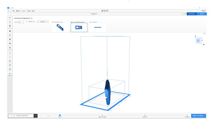
**MAX. PLATFORM CONTACT\*** - this position arranges the biggest flat surface of a model directly on the platform. Thanks to that the model will adhere better to the platform.
