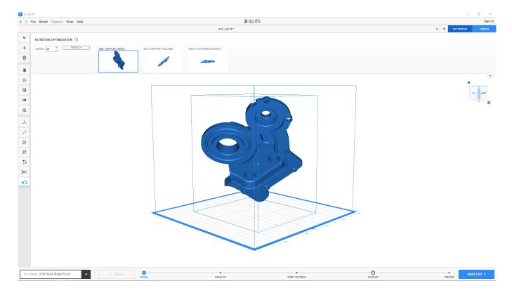
**MIN. SUPPORT AREA** – this position reduces the number of required support structures. It means that the need of further mechanical treatment is minimized and there are fewer marks on the model's surface after removing the support.
