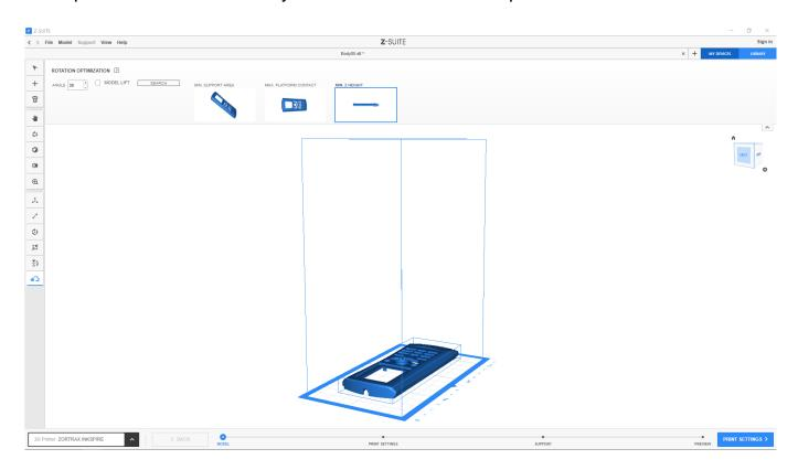
**MIN. Z HEIGHT** - this position arranges a model horizontally on the platform. In this way it is possible to significantly speed up the printing process.
