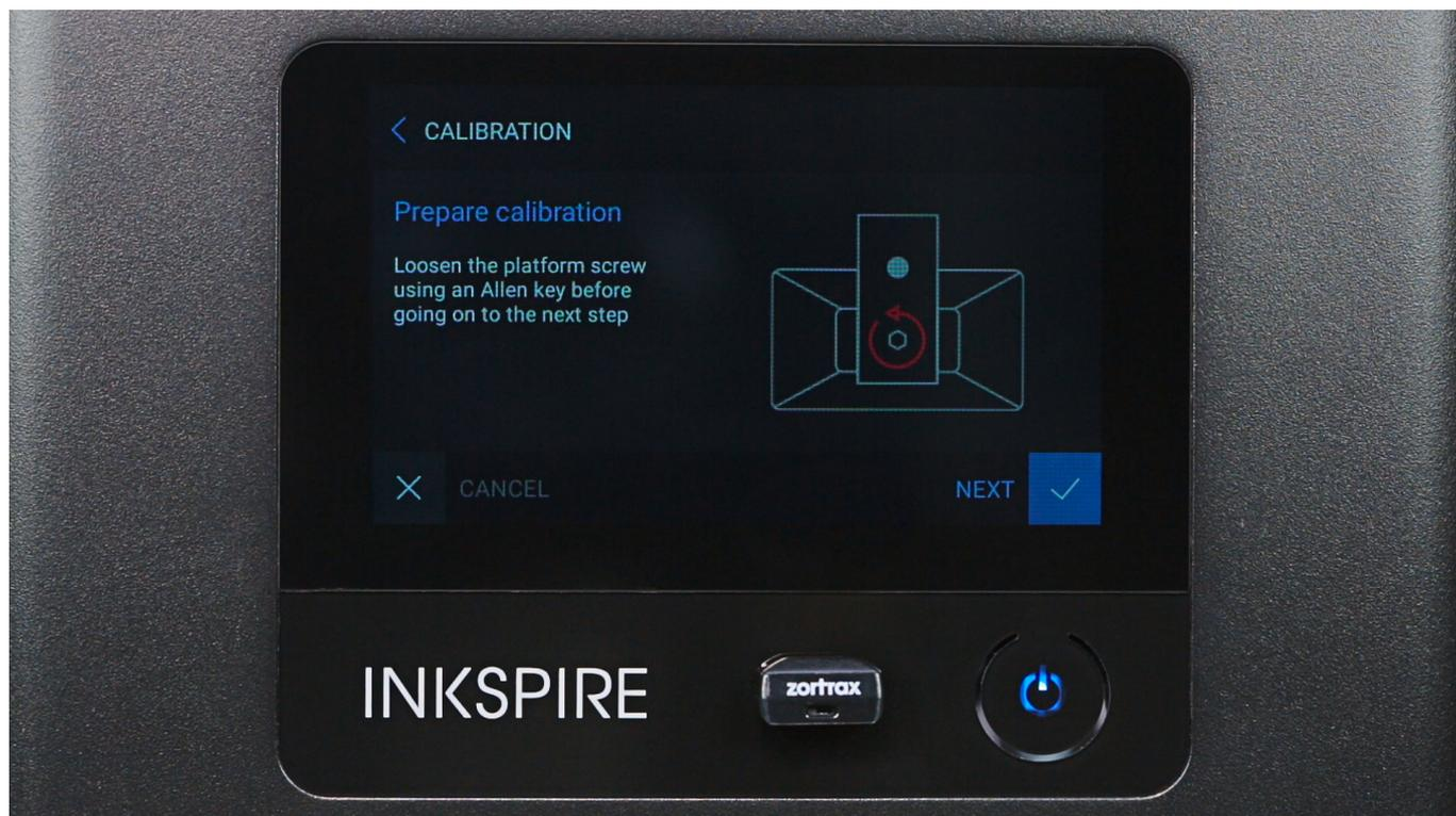
Loosen the platform screw with an Allen key. Tap *Next* to continue.
