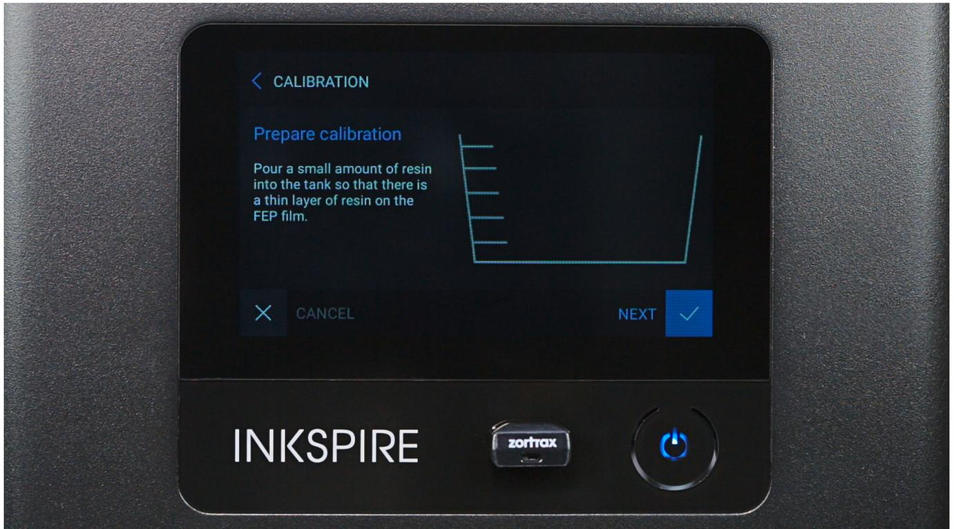
Pour a small amount of resin into the tank so that there is a thin layer of resin on the FEP film. Tap *Next* to confirm.
