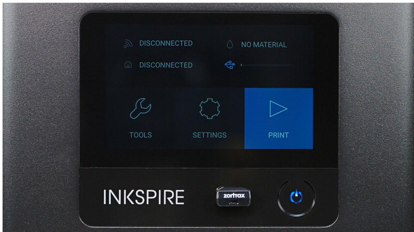
Start the calibration with the options from the menu. Select *Tools* and then *Calibration*. At this point the printer will start to lift up the platform.
