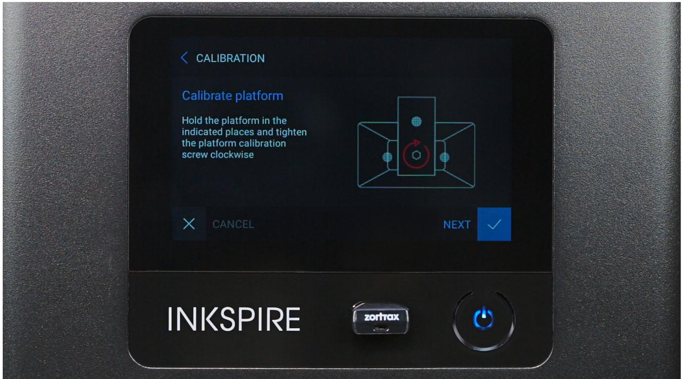
Hold the platform block in the places shown in the video and press the platform against the screen. Next, tighten the platform screw. Install the UV cover back on the printer.
