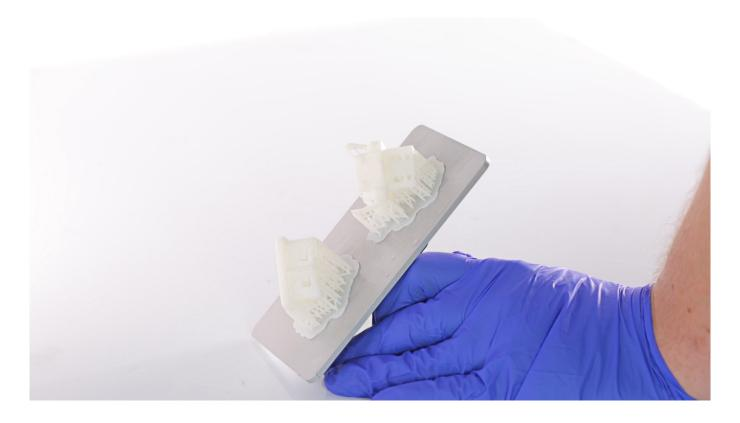
Remove the model from the platform by hand or use a spatula. If you have problems with removing the print, use a cutting knife.
