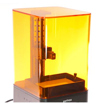
Remove the UV cover. Install the platform back in the printer and secure it with the screw.
