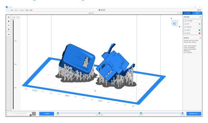
Once you finish preparing the file, transfer it from Z-SUITE to the printer's storage (via Wi-Fi/Ethernet cable) and start the printing process.
