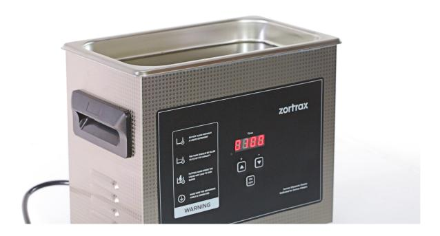
Immediately put the platform with the model in the Ultrasonic Cleaner and turn on the device.
