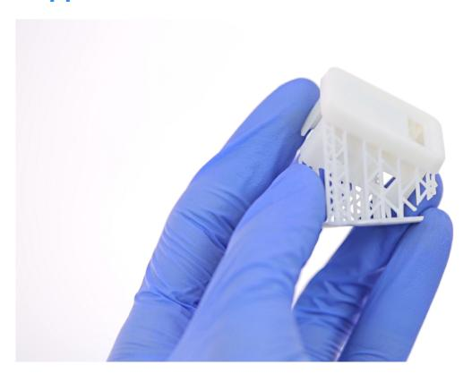
Remove the raft and support structures from the model.
