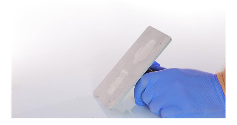
Clean the platform surface with a spatula to remove residues of cured resin. Next, put the platform in the Ultrasonic Cleaner and turn on the device for about 30-60 seconds.
