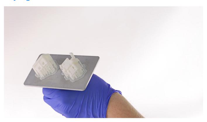
Leave the platform with the model to air dry and ensure that the model isn't exposed to the UV light until it's completely dry. You can use compressed air for better and faster drying.
