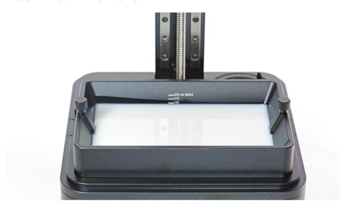
Unscrew the two screws that secure the resin tank and remove them. Next, remove the resin tank.
