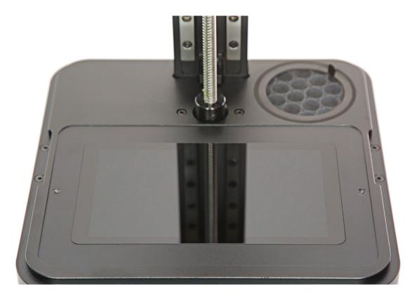
Install the resin tank in its place and tighten the two screws.
