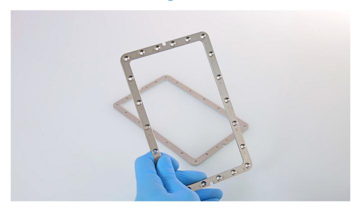
Clean both parts of the FEP film rack with a paper towel soaked in isopropyl alcohol.
