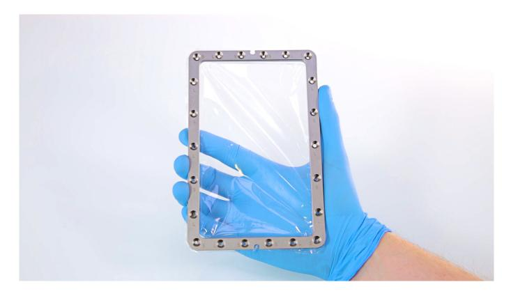
Separate both parts of the rack and remove the FEP film.
