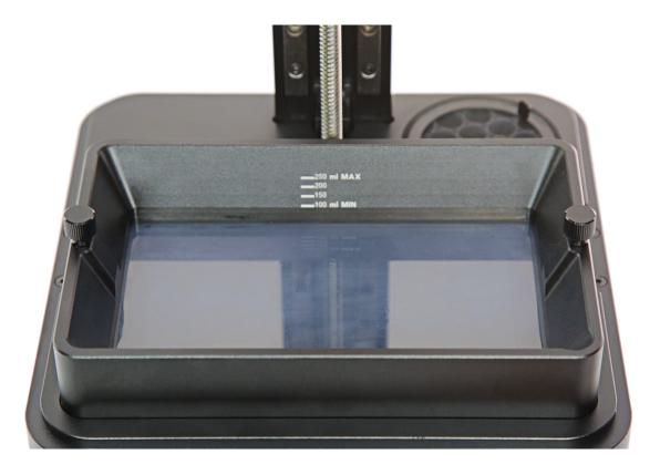
Loosen the two screws that secure the resin tank. Next, remove the tank.
