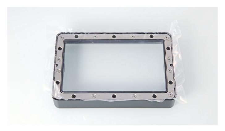
Cut and remove the excess FEP film from the rack.
