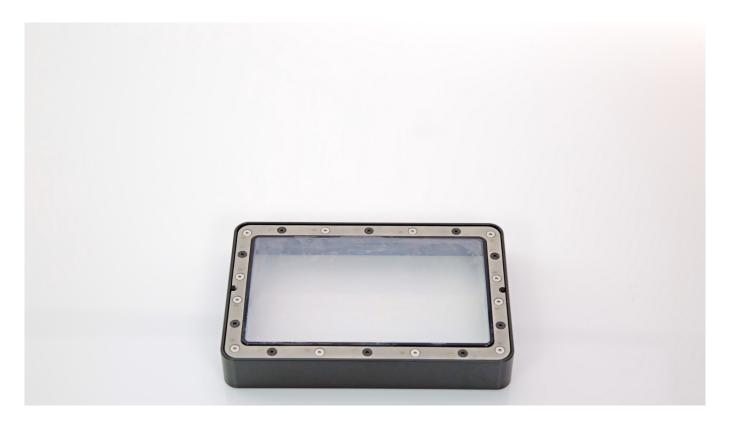
Unscrew the black screws that secure the FEP film rack to the resin tank. Next, separate the FEP film rack from the resin tank.
