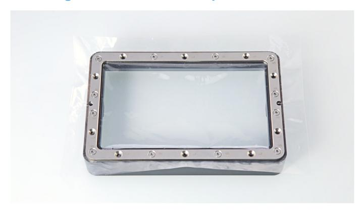
Secure the FEP film rack with the black screws in a diagonal order. Once you finish, fully tighten all screws.
