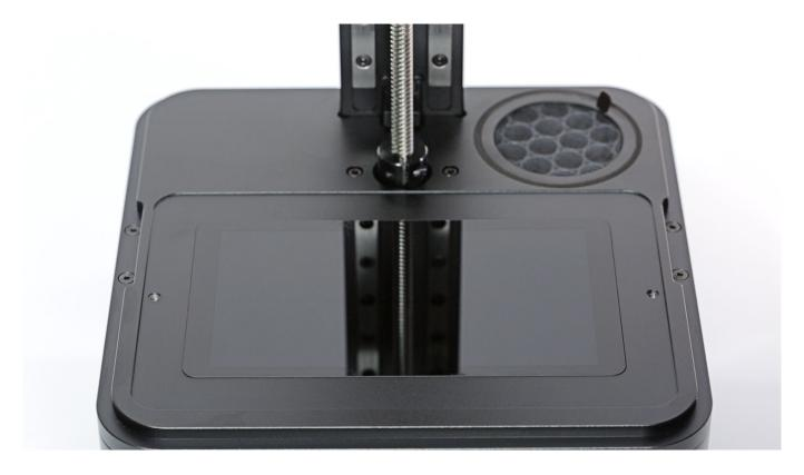
Install the resin tank in its place and tighten the two screws.
