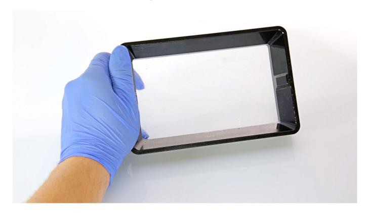
Clean the resin tank with a paper towel. You can also use 99% isopropyl alcohol for that purpose. If you change the color or type of resin, clean the tank in the Ultrasonic Cleaner.
