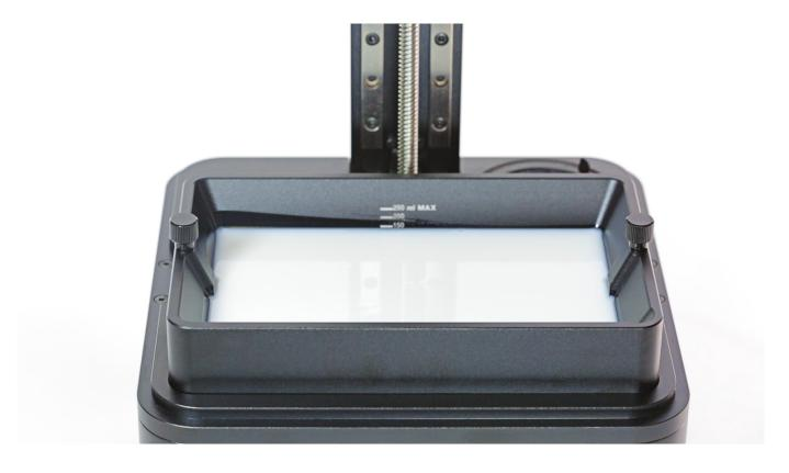
Loosen the two screws that secure the resin tank. Next, remove the tank.
