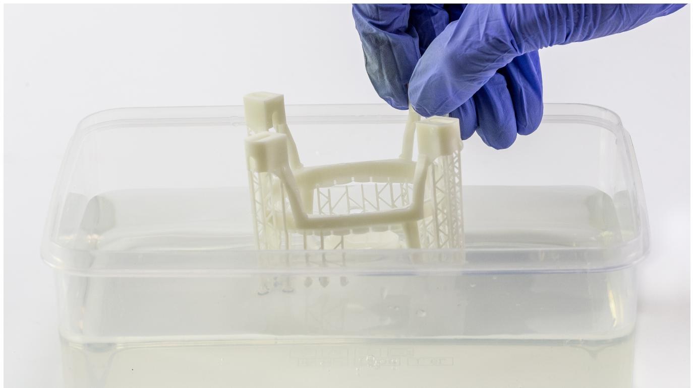
Remove the model from the box and protect it from UV light until it is dry.
