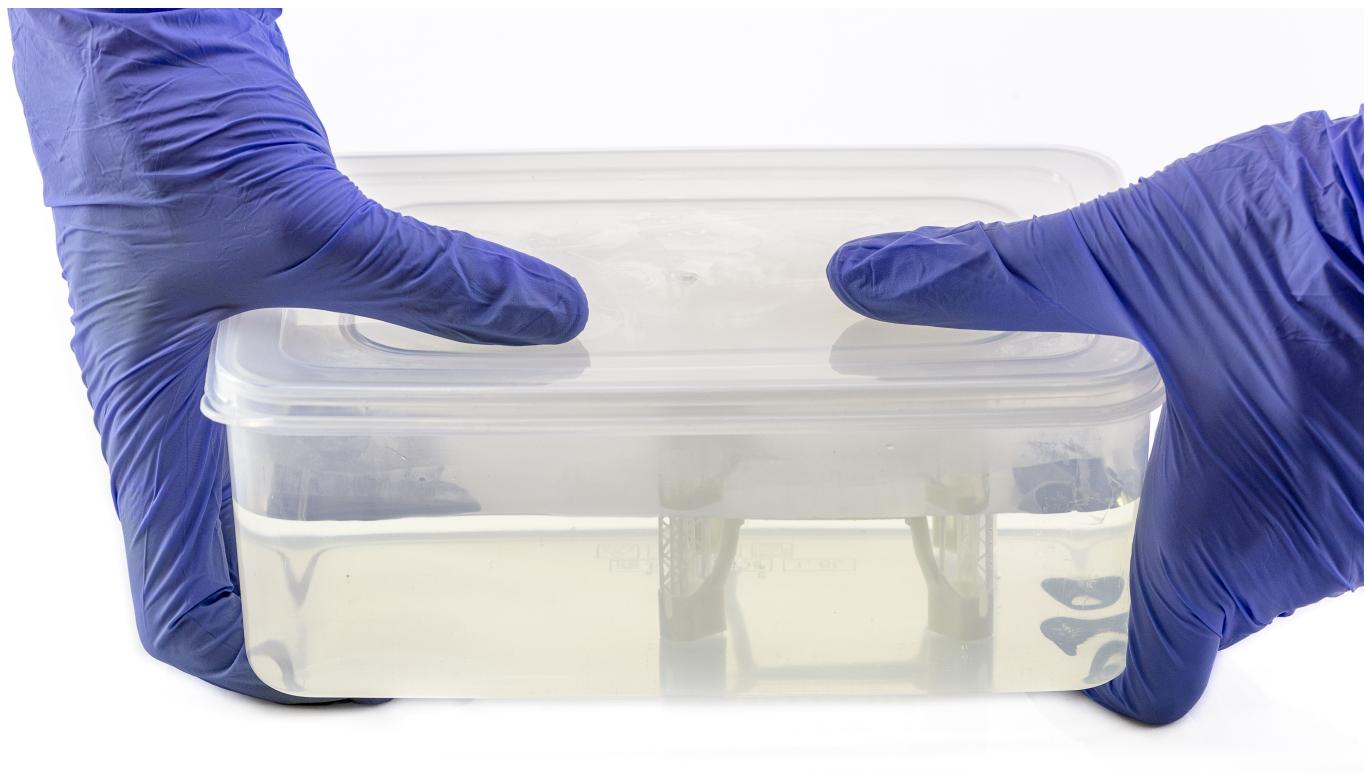
Clean the model from liquid resin by slightly shaking the box.
