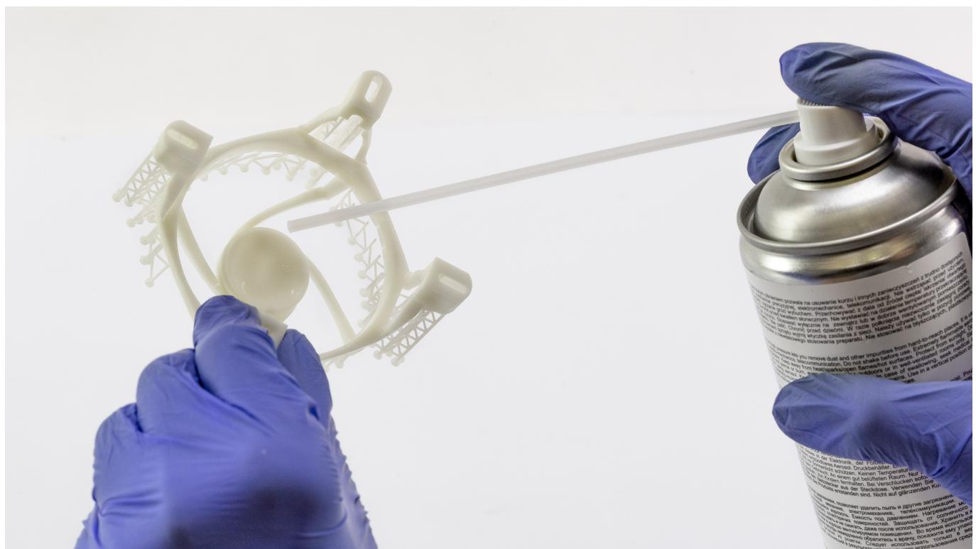
Use compressed air to remove liquid remains from the model.
