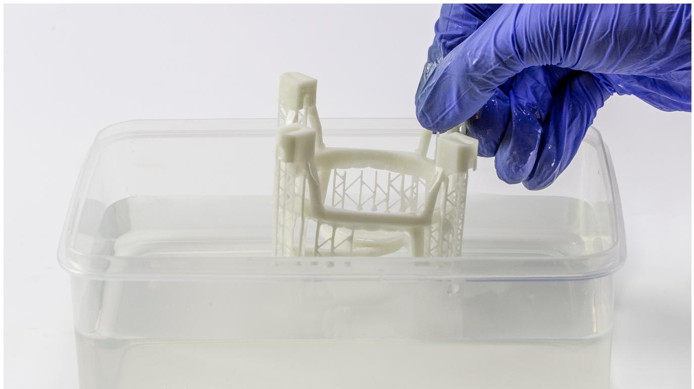
Fill up the cleaning box with a liquid detergent (isopropyl alcohol can be used). Put the
