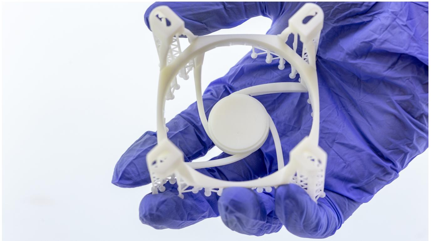
Leave the model to air dry. The model can be cured in UV light once it is completely dry.
