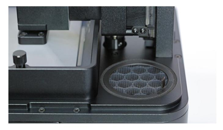
Remove the filter from the printer's housing.
