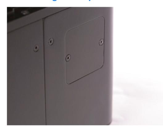
Unscrew the two screws that secure the inspection hatch cover. Next, remove the cover using the adhesive piece.
