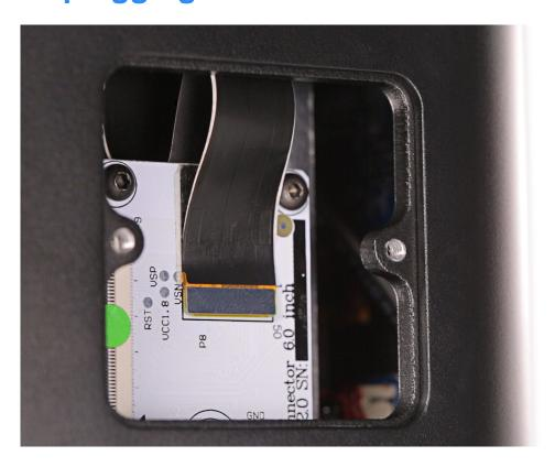
Use tweezers to unplug the LCD screen cable from the PCB.
