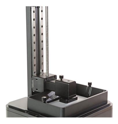
From the menu select "Tools," "Platform" and "Move the platform." Keep the UP arrow pressed to lift the platform.
