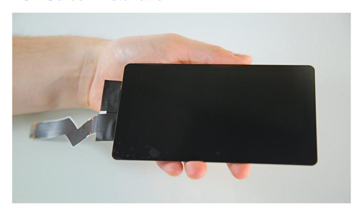
Carefully remove the protective foils from the new LCD screen. Next, pass the screen cable through the slot in the housing. Use tweezers to take out the cable from behind the PCB. Install the screen in its place.
