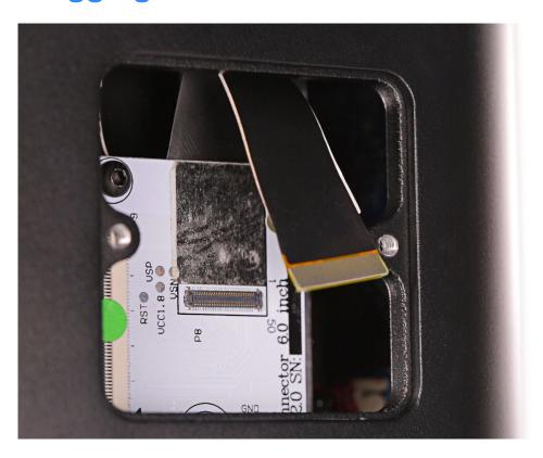
Plug the LCD screen cable into the PCB.
