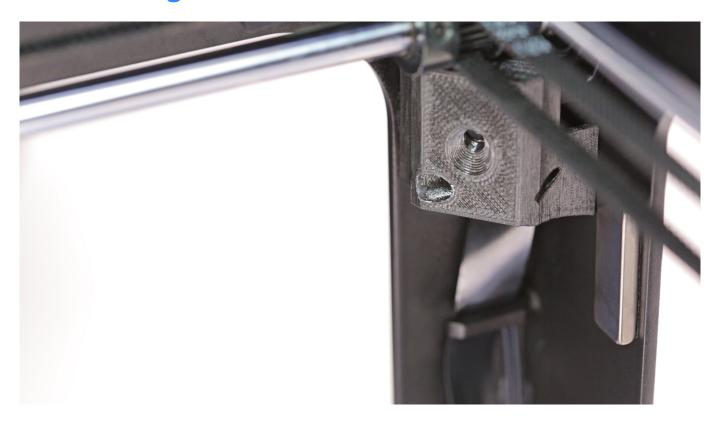
Unscrew one screw that secures the camera in the printer's frame. Use a 2mm Allen key.
