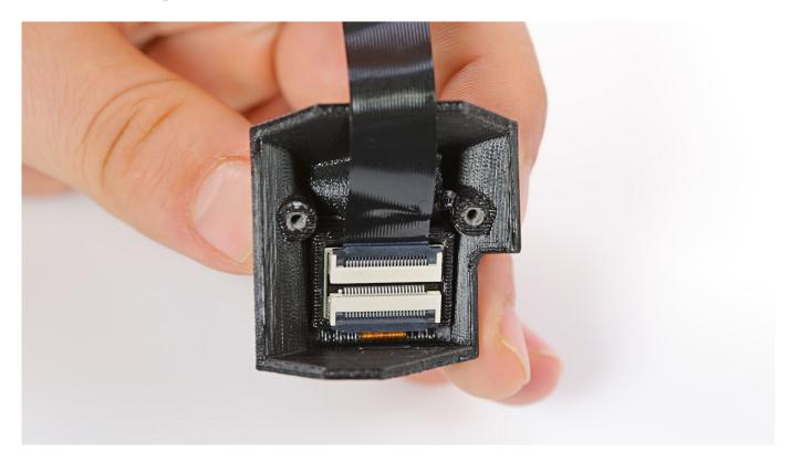
Separate the camera from its printed case.
