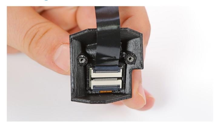
Separate the camera from its printed case.
