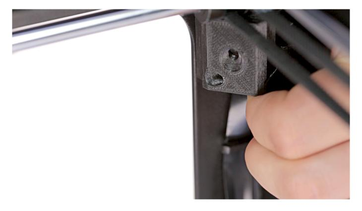
Remove the camera together with its cable from the printer's frame.
