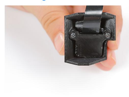
Unscrew the two screws that secure the camera's back cover. Use a Phillips screwdriver.
