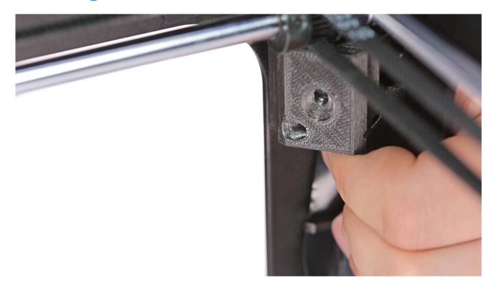
Secure the camera to the printer's frame with the screw.
