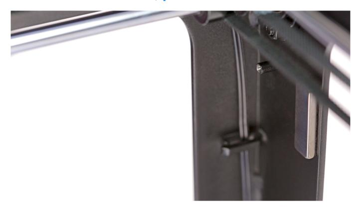
Install the camera with its cable in the printer's frame.
