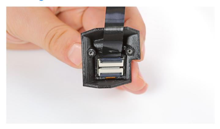
Secure the camera's back cover with the two screws.
