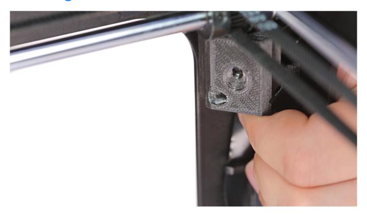
Secure the camera to the printer's frame with the screw.
