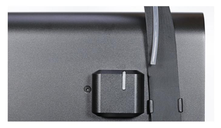
Attach the material guide to the endstop.
