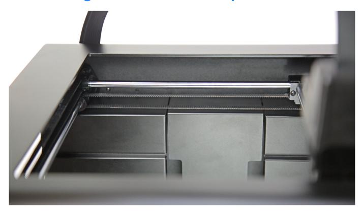
Unscrew one screw that secures the material endstop in the printer's frame.
