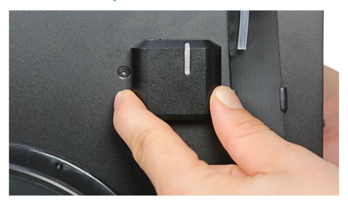
Remove the material endstop from the printer's frame. Unplug the endstop cable.
