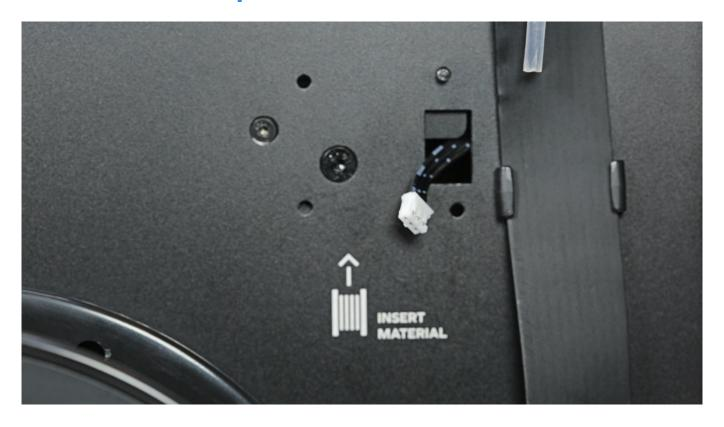
Prepare the new material endstop and plug in the cable. Attach the endstop to the printer's frame.
