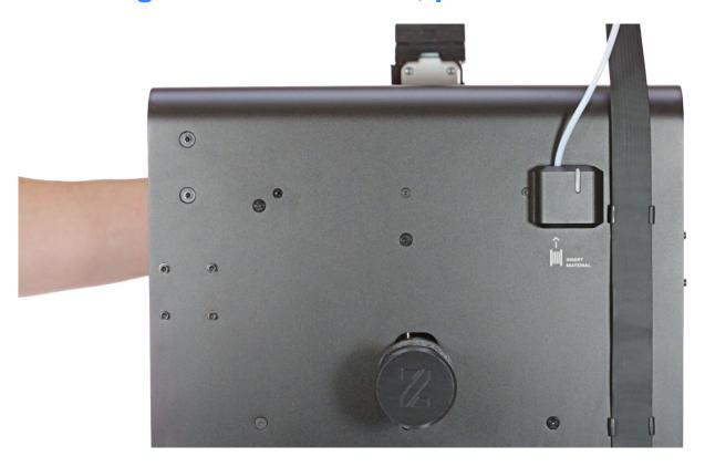
Secure the cover by fixing the screw at the back of the printer.
