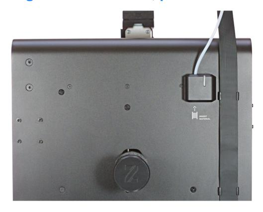
Unscrew the screw that secures one part of the Z-axis cover at the back of the printer.
