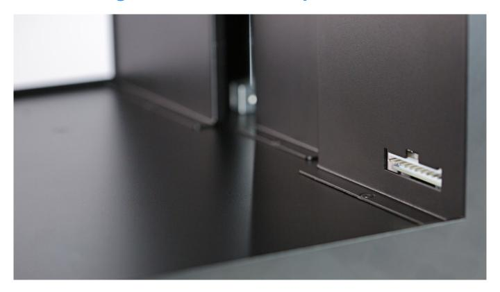
Unscrew the screw that secures one part of the Z-axis cover inside the printer.
