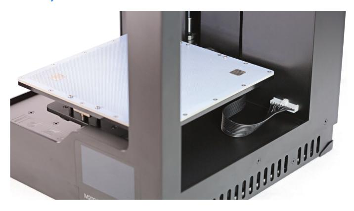
Unplug the heatbed cable from the Z-axis cover.
