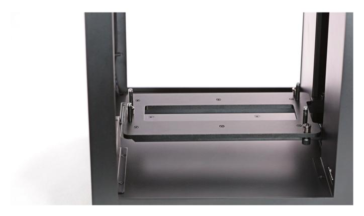
Place the heatbed cable behind the heatbed mount and install the platform back in the printer.
